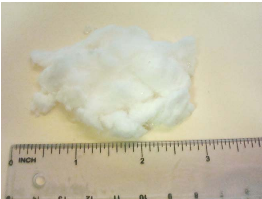
Figure 1 – Optical photograph of as-formed 93B3 fibers (300nm to 5 \mu m diameter).
