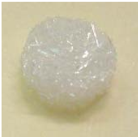
Figure 1 – Image of a 13-93 random fiber scaffold. The scaffold measures 7mm in diameter and 2mm thick and has an open porosity of 50% and a compressive strength of 5MPa.
