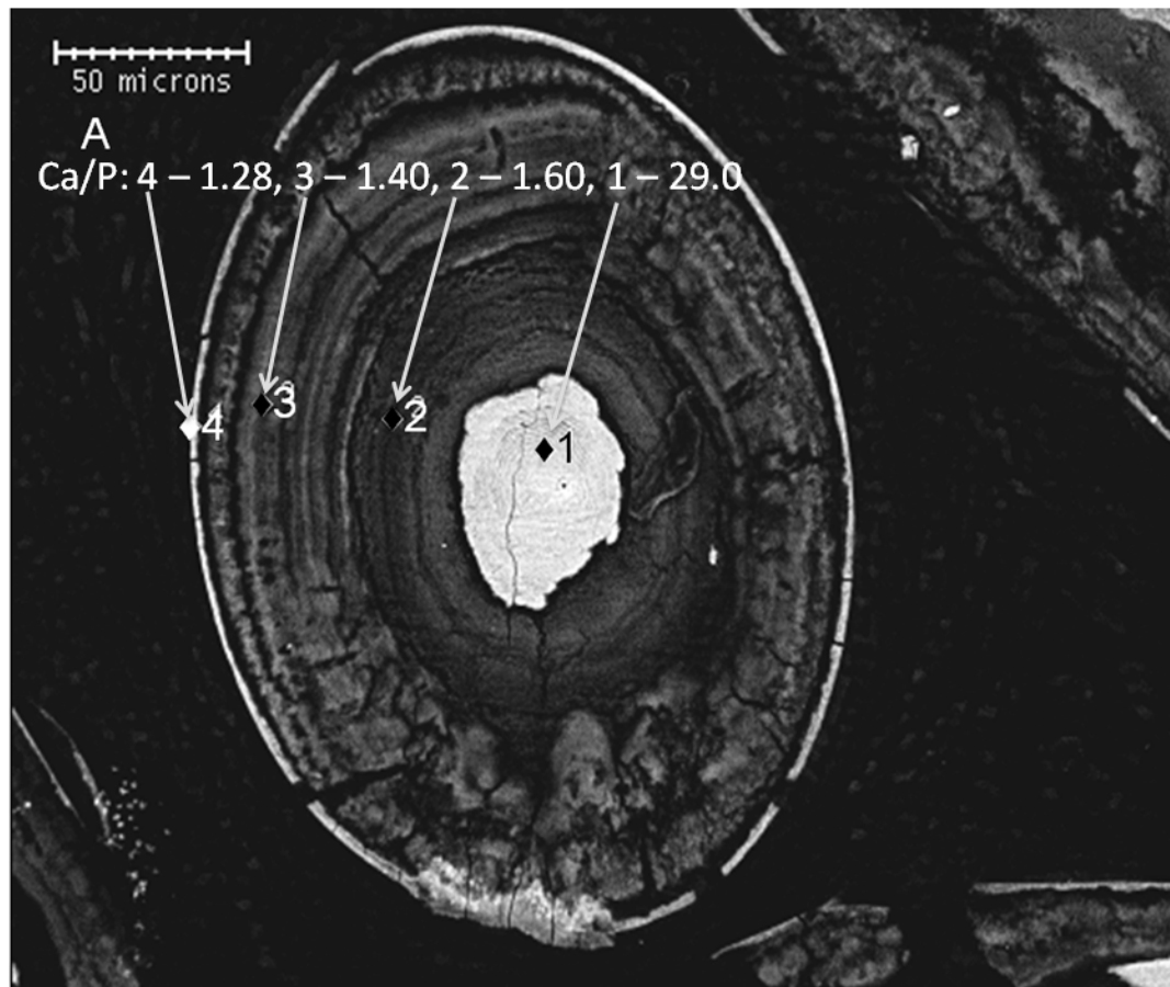
Figure 19 - SEMBSE image of a CSZF fiber implanted subcutaneously in a rat for six weeks.
