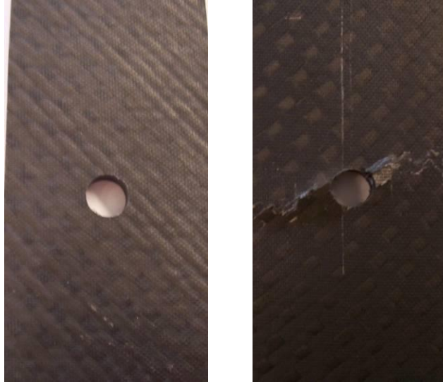
Figure 24. Cycom 977-20/AS4-5HS Carbon Composite Specimens Before (Left) and After OHC Testing (Right)
