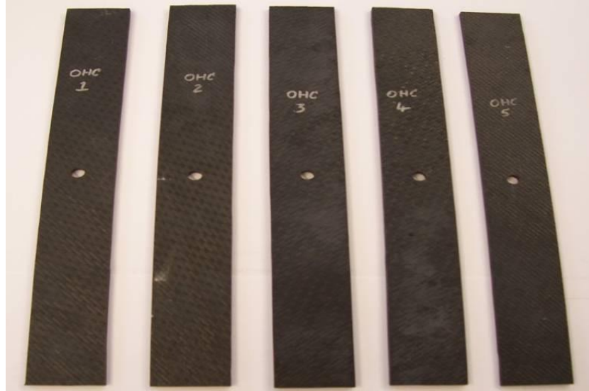
Figure 22. OHC Testing Coupons of Cycom 977-20/AS4-5HS Carbon Composites
