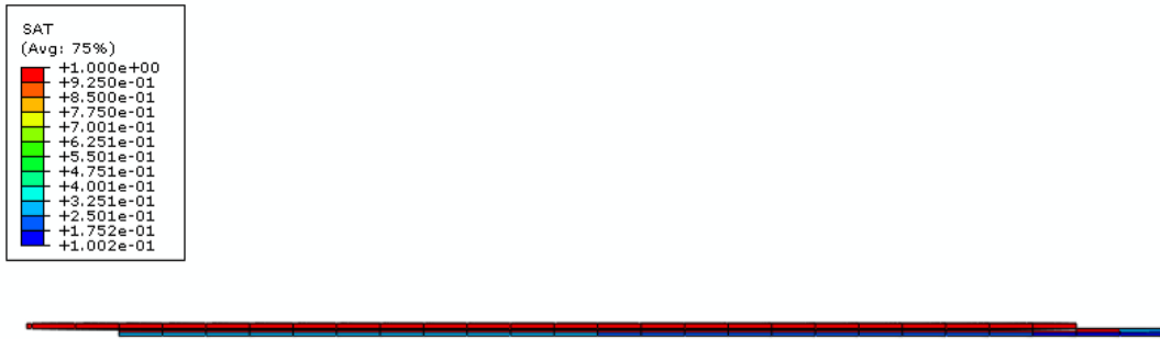
Figure 33. Saturation Distribution of Cross-section at Time = 225 sec
