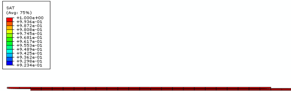
Figure 34. Saturation Distribution of Cross-section at Time = 435 sec
