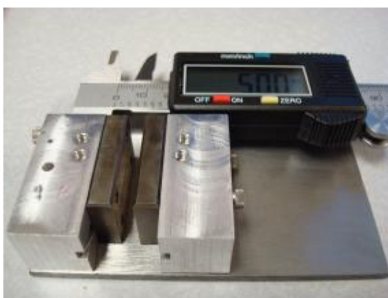
Figure F.1. Two-point bend apparatus design for Raman spectroscopy.
