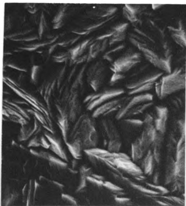
FIGURE 18. SCANNING ELECTRON MICROGRAPHS OF A DEPOSIT PRODUCED AT 50°C WITH GRAPHITE ANODES (upper) AND DEPOSITS PRODUCED AT 30°C WITH VITREOUS CARBON ANODES (lower).
