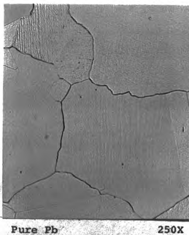
FIGURE 2. MICROSTRUCTURES OF THE AS ROLLED SURFACE OF LEAD AND LEAD ALLOYS USED IN THIS WORK.
