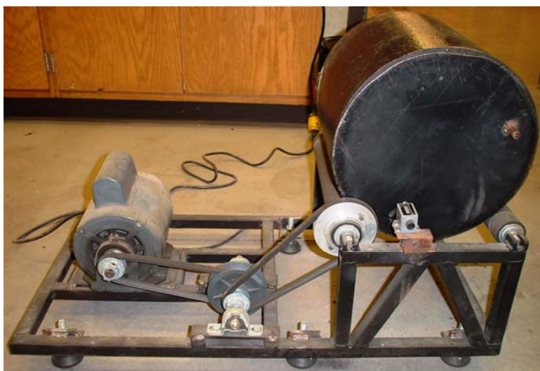
Figure 3. 12"x12" end-loading (opposite face) smooth ball mill on stand for Bond closed-circuit grindability test.
