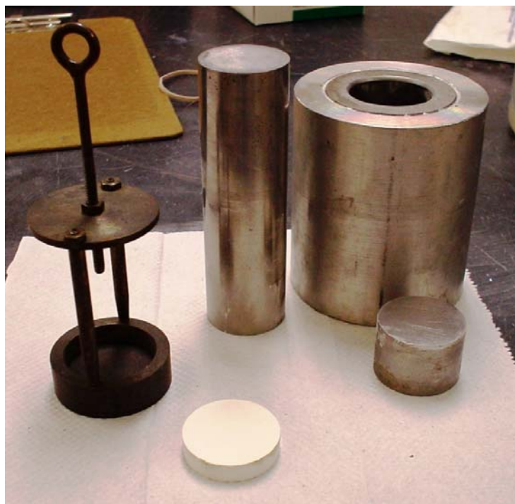
Figure 2.5. Sample holder (left), pressed sample disc of CaO (middle bottom), and Carver press ram with cylinder (back right) used to make samples for TGA reactor
