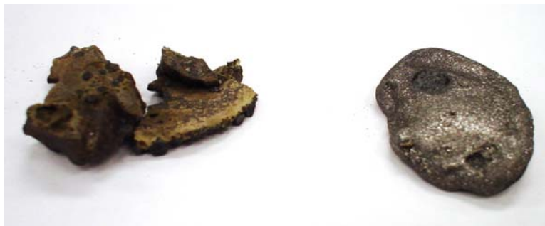
Figure 5. Mechanical separation of slag (left) and metallic (right) fractions after inert induction melting and cooling.
