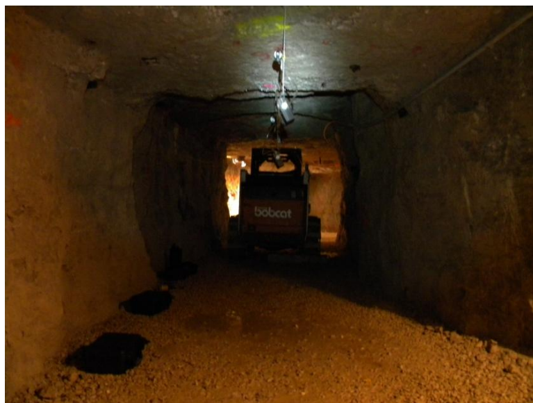
Figure 5.5. Layout of the Experiment: Bobcat loader Put in Fixed Position and Four SKC DPM Sampling Trains Located Downstream of the Exhaust Pipe
