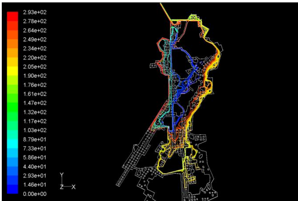
Figure 6.3. Path of Small Particles without Stoppings
