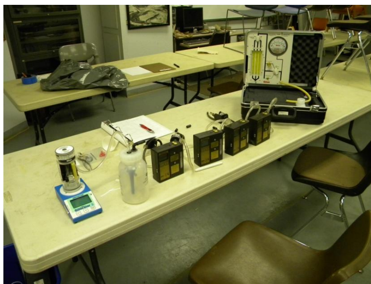
Figure 5.4. Calibration of the Sampler Pump before the Experiment
