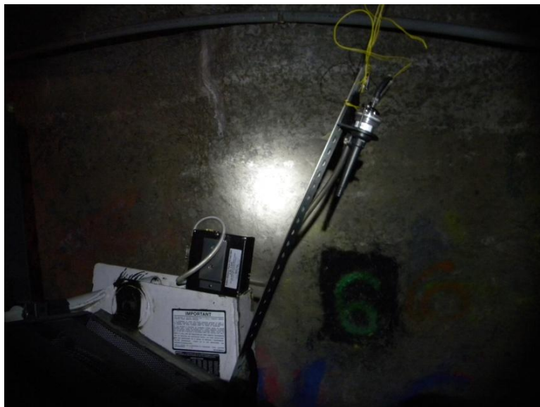
Figure 5.6. Installation of the Sampling Train Close to the Tailpipe
