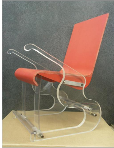
Figure 1.1. An Ergonomic Modular Compliant Chair in its Undeformed State
