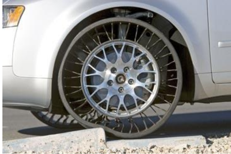
Figure 1.11. Michelin Tweel™ Airless Tire [5]
