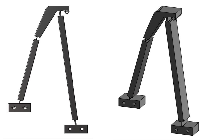
Figure 6.4 Solid Model of the Compliant Mechanism Designed in Example 1
