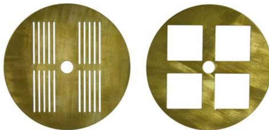
Figure 2 – Machined brass shadow masks for electrode (left) and dielectric (right) patterning. The use of the electrode mask results in a capacitor area of 2.56 \times 10^{-2} \text{ cm}^2 .
