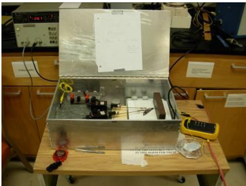
Figure 8 – Image of the specially made, solid Al Faraday cage used for a portion of the electrical testing.
