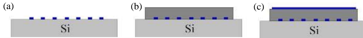
Fig. 1 – Process sequence followed for the patterned deposition of a single dielectric layer capacitor. 1 st electrode layer (a), dielectric (b), and 2 nd electrode layer (c). Layer thicknesses are proportioned approximately for 25 nm thick Ni with 150 nm thick BaTiO 3 . Vacuum was broken between layers to allow the exchanging of physical masks between depositions.
