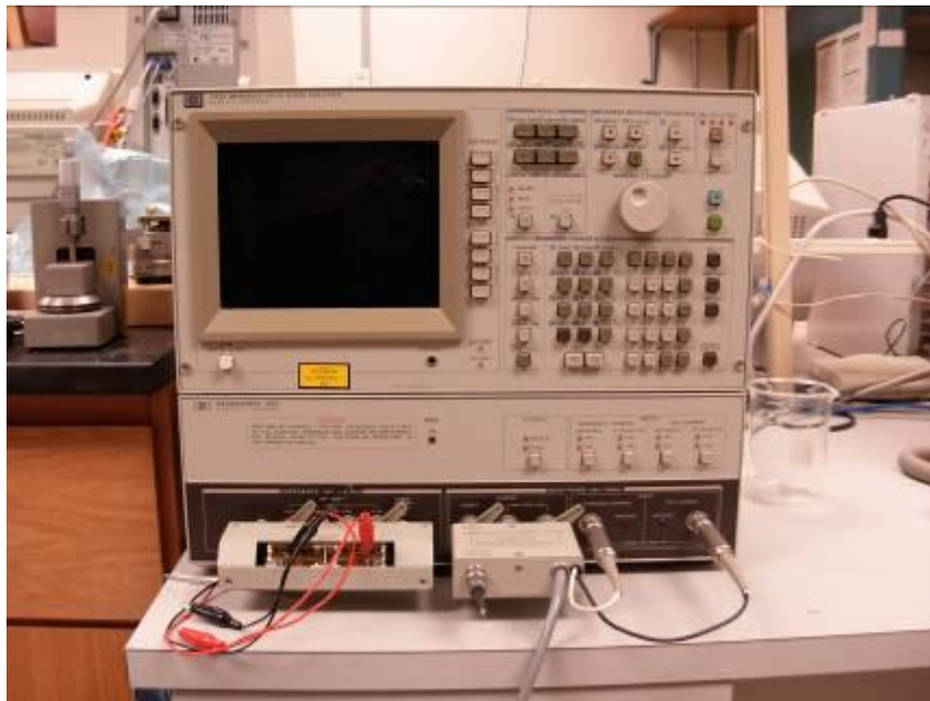
Figure 7 – The HP 4194 used for more in depth AC characterization at 1 V_{\text{rms}} with 0 V DC bias at frequencies between 500 and 200,000 Hz.
