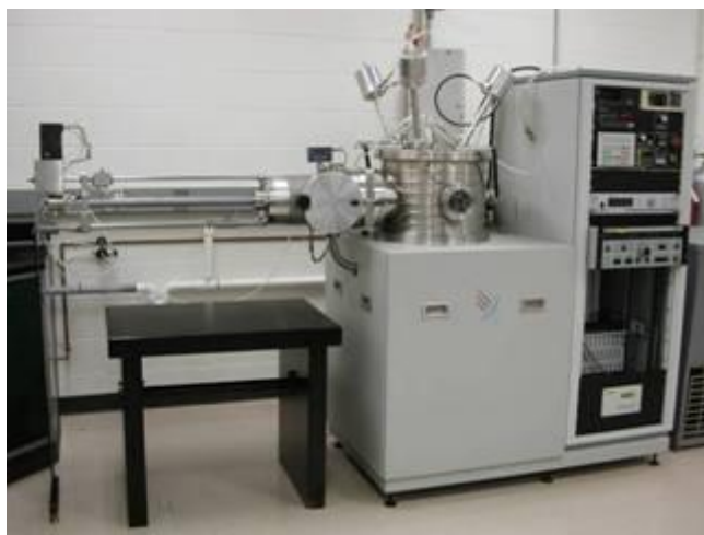
Figure 1 – Photograph of Denton Discovery-18 Sputter Deposition System used for this research.
