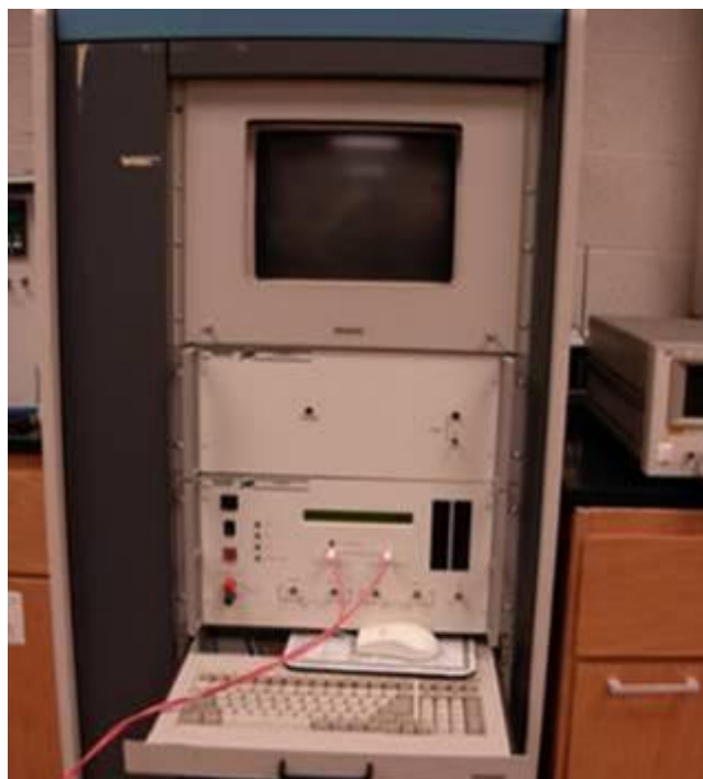
Figure 5 – The Radiant Technologies RT6000HVS used for the acquisition of hysteresis loops for the sputtered BaTiO 3 capacitors.
