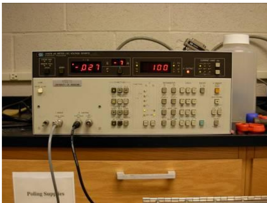
Figure 4 – The HP 4140 pA Meter used for the acquisition of I-V plots from the sputtered BaTiO 3 capacitors with either Ni or Pt electrodes.
