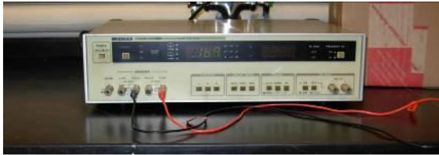
Figure 6 – The Leader LCR-745-01 test bridge used for initial AC investigations at 1 kHz, 1 V_{\text{rms}} , and 0 V DC bias.
