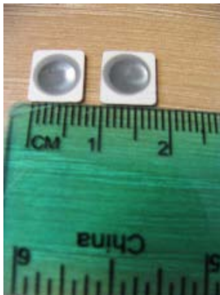
Fig. 2.19. Dimpled glass ceramic dielectric composition prepared from G-0175.
