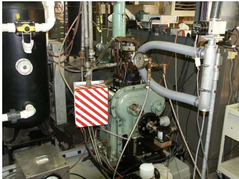
Figure 2.2. CFR engine setup
