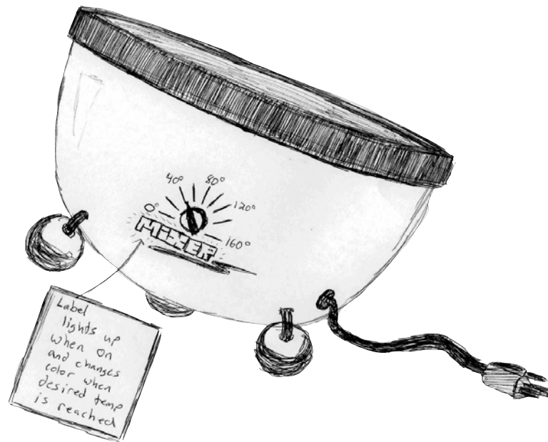
Figure 6.16. Solution sketch generated from the morphological matrix shown in Figure 6.15 for the drink mixer redesign scenario. Highlighted solutions shown in Figure 6.15 were used to produce this complete conceptual design.
