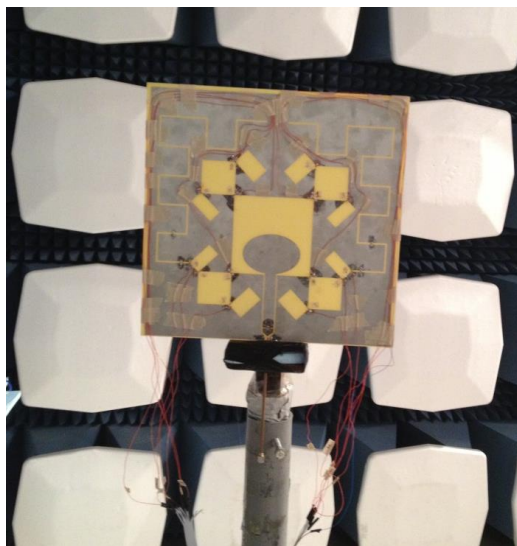
Figure 6.38. Antenna Design 3 with all the PIN diodes and DC bias lines installed (placed on a stand inside anechoic chamber).
