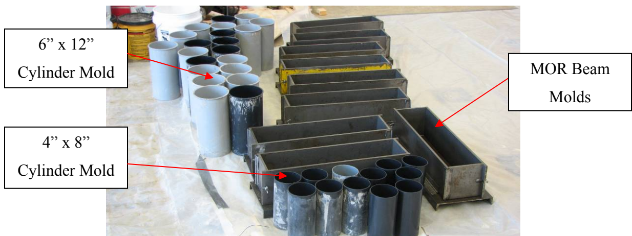
Figure 3.20 Auxiliary Specimens for Concrete Material Testing
