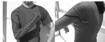
Figure 9: Printed piezoresistive sensor for wearer [15]
