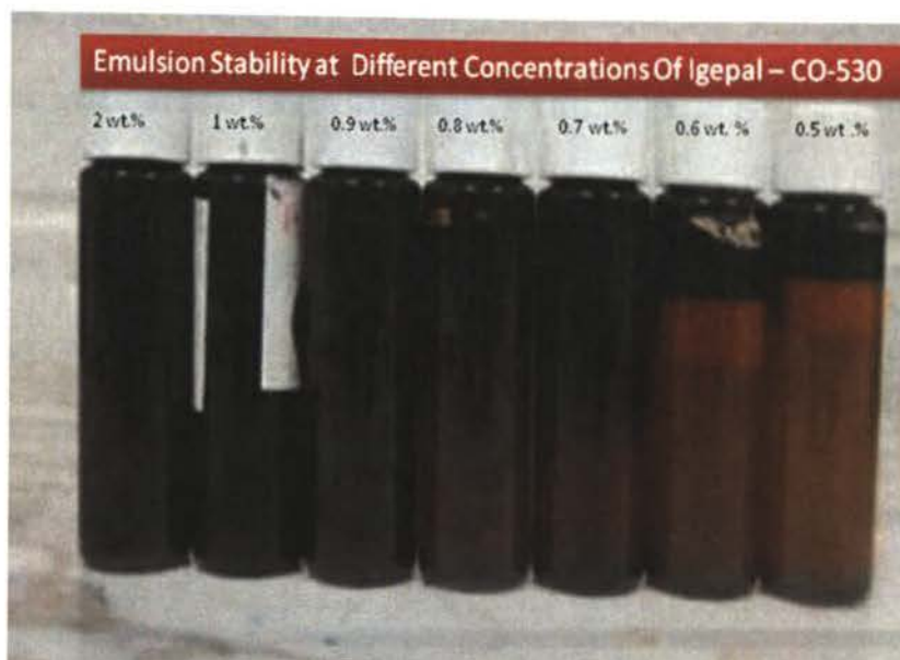
Figure 3.17 Effect of Surfactant Concentration on Emulsion Stability
