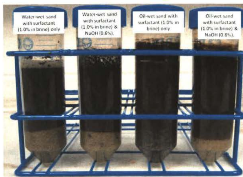
Figure 3.20 Effect of Igepal CO-530 and Alkaline NaOH on Wettability
