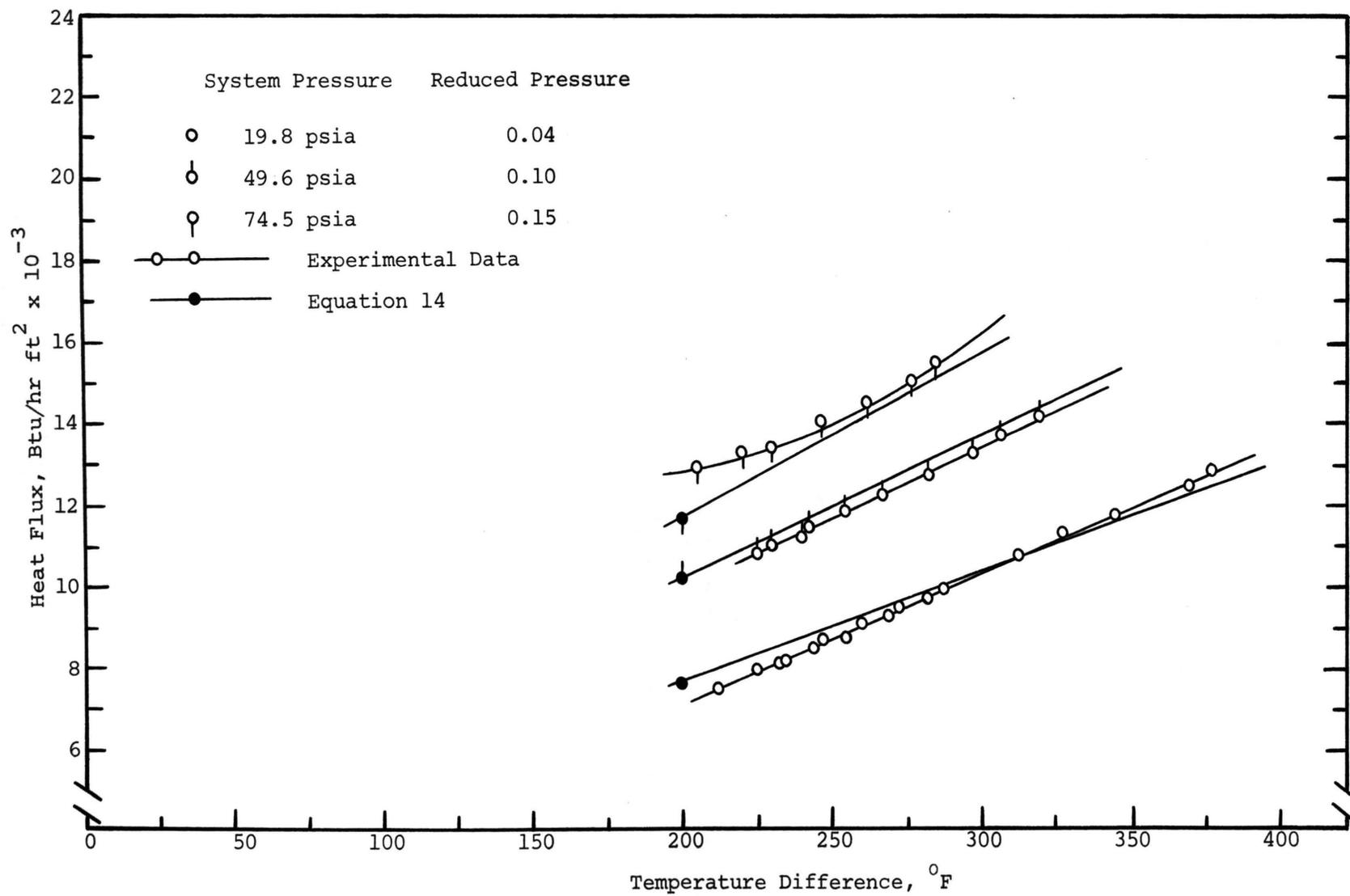
Figure 28. Film Boiling Comparison with Equation 14, Freon 113, 1.00 Inch Surface
