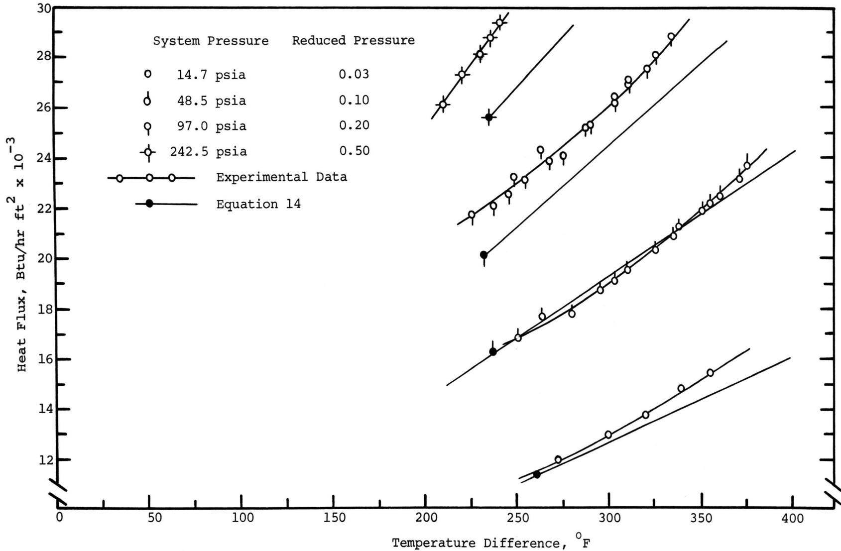
Figure 25. Film Boiling Comparison with Equation 14, n-Pentane, 1.00 Inch Surface
