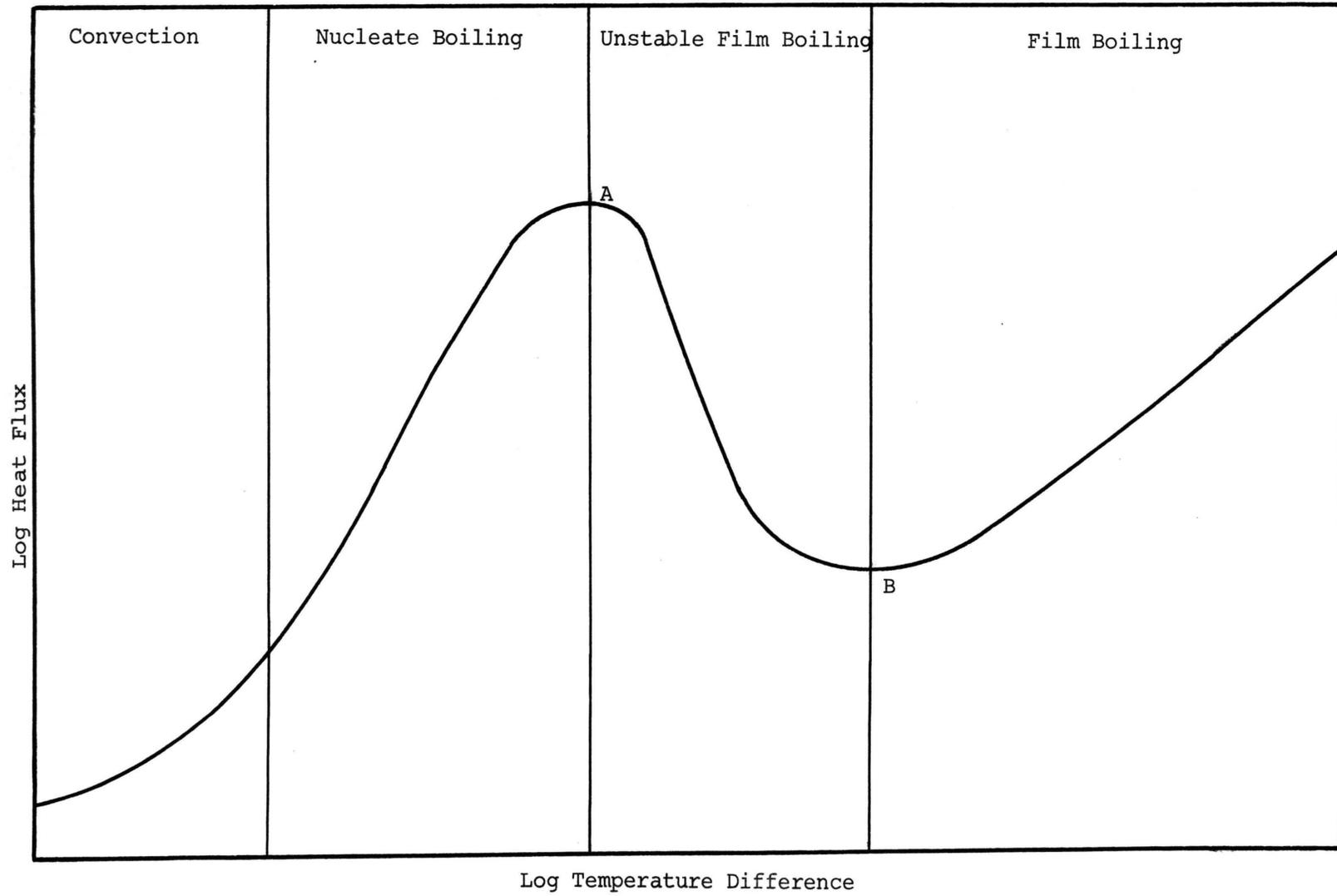
Figure 1. A Typical Boiling Heat Transfer Curve
