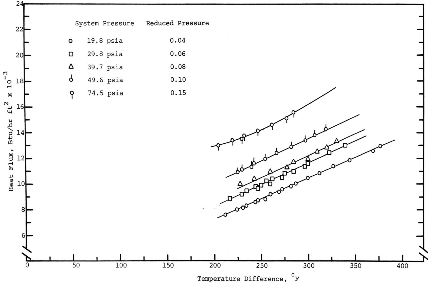
Figure 4. Film Boiling Results of Freon 113, 1.00 Inch Surface
