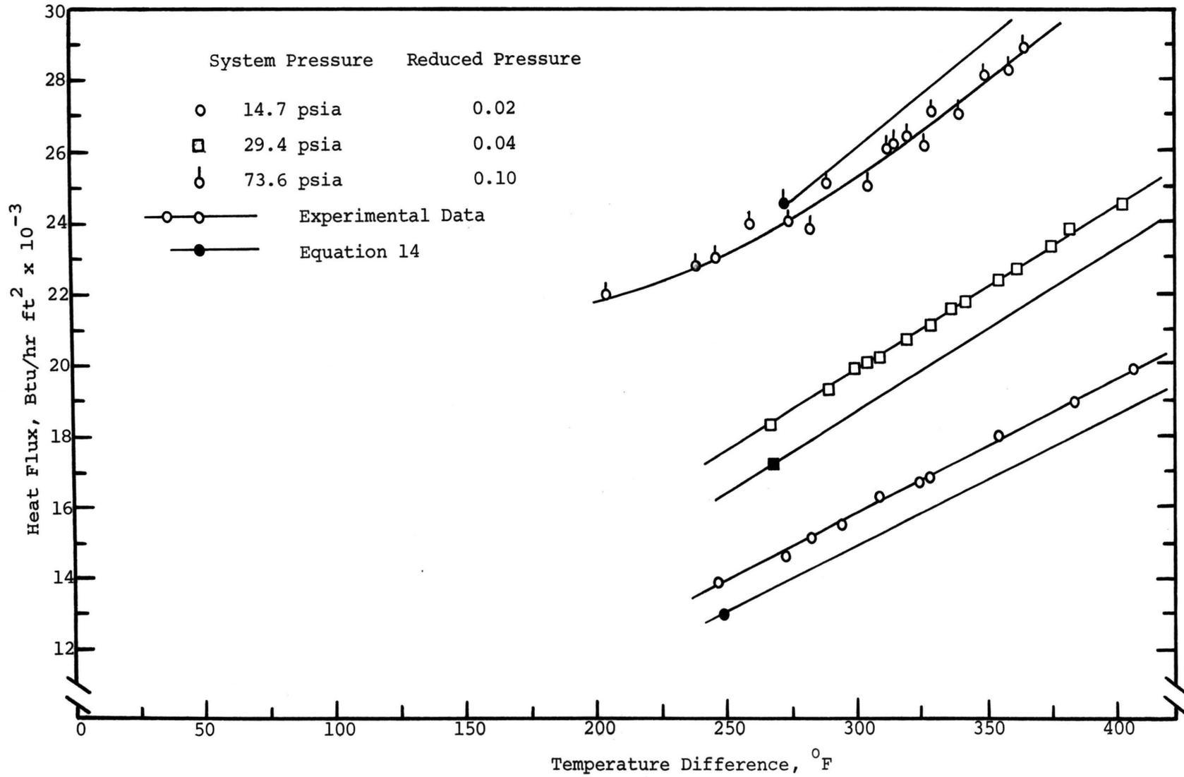
Figure 31. Film Boiling Comparison with Equation 14, Benzene, 1.00 Inch Surface
