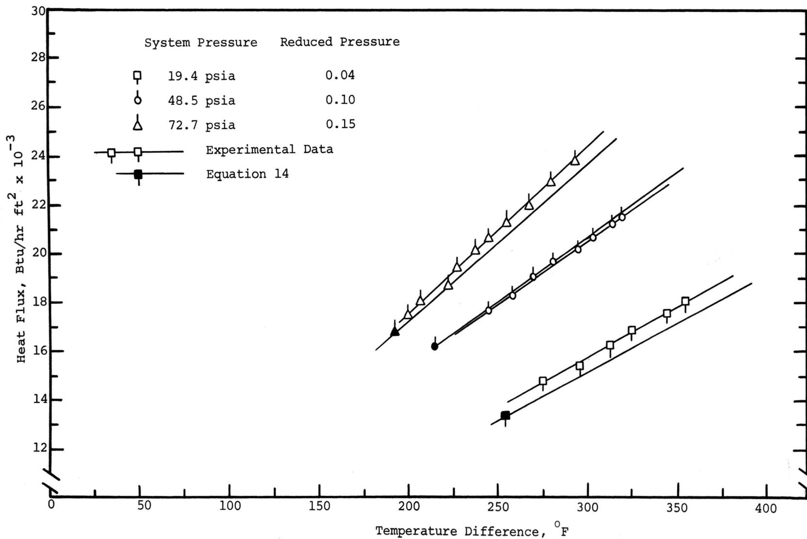
Figure 27. Film Boiling Comparison with Equation 14, n-Pentane, 0.75 Inch Surface
