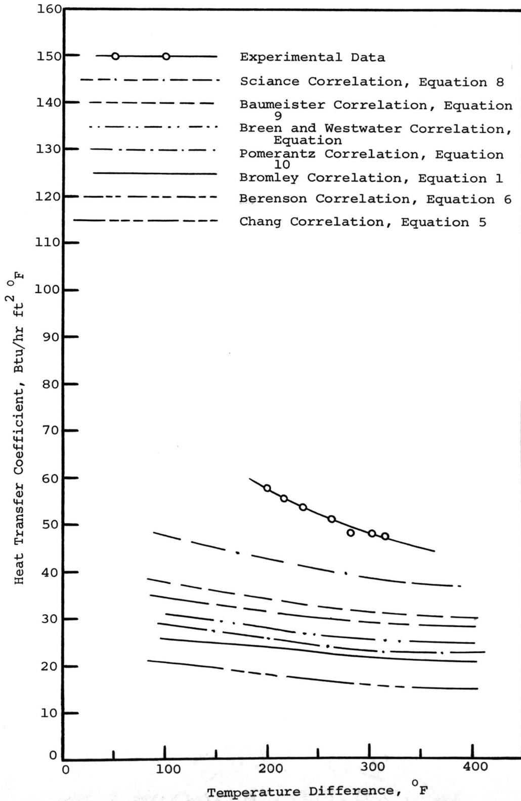
Figure 22. Comparison of Film Boiling Correlations, Freon 113, 49.5 psia, 0.55 Inch Surface
