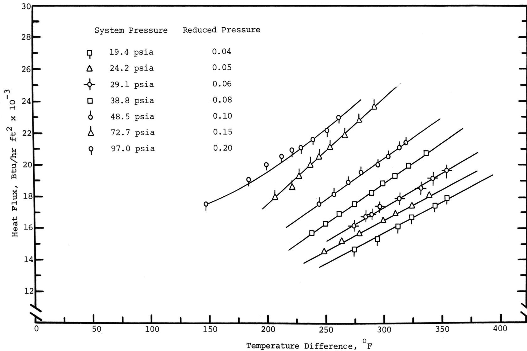
Figure 8. Film Boiling Results for n-Pentane, 0.75 Inch Surface
