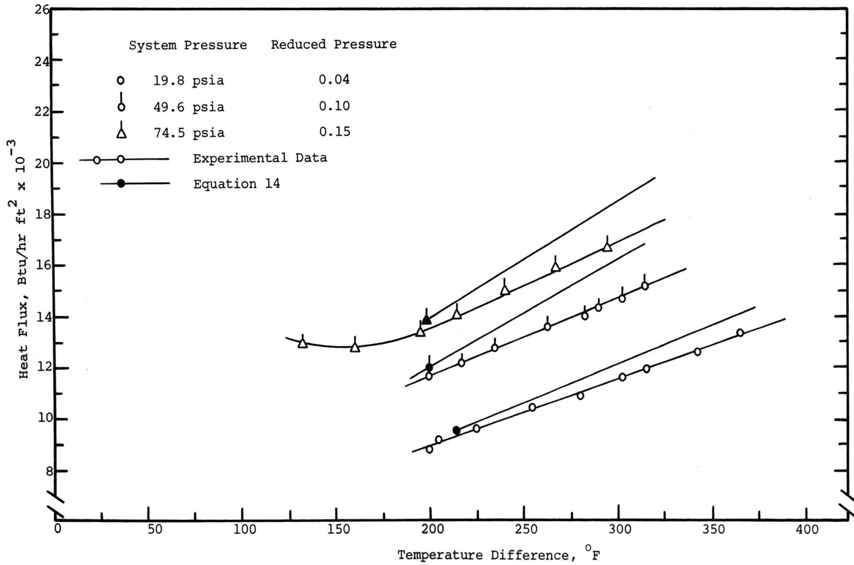
Figure 30. Film Boiling Comparison with Equation 14, Freon 113, 0.55 Inch Surface
