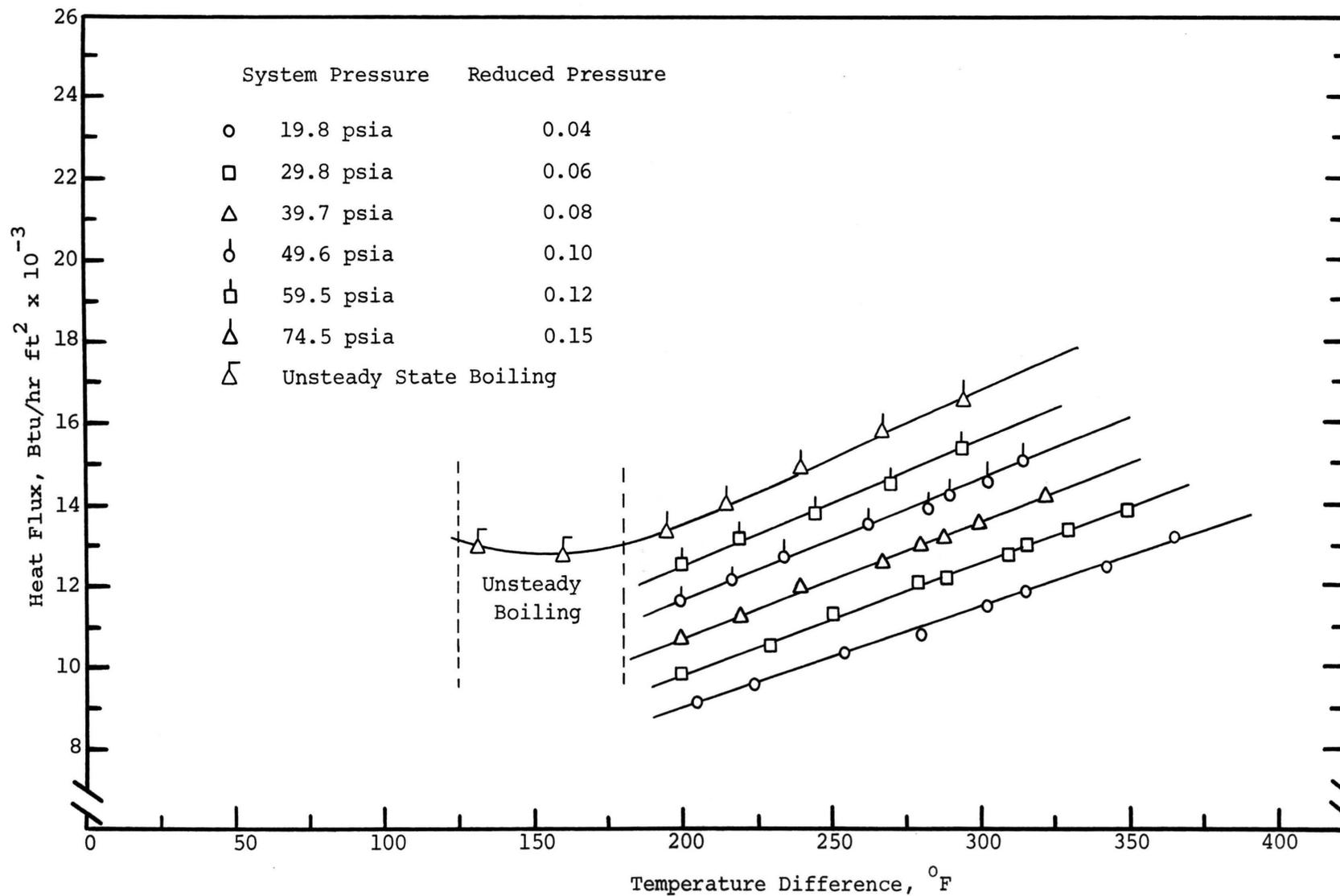
Figure 6. Film Boiling Results for Freon 113, 0.55 Inch Surface
