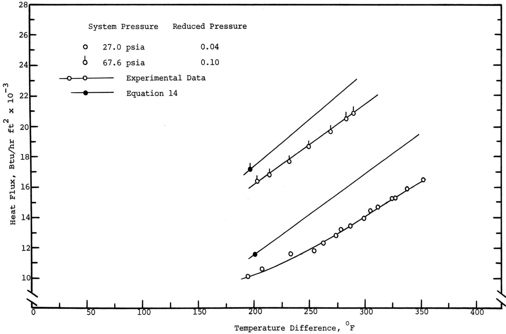
Figure 32. Film Boiling Comparison with Equation 14, Cyclopentane, 1.00 Inch Surface
