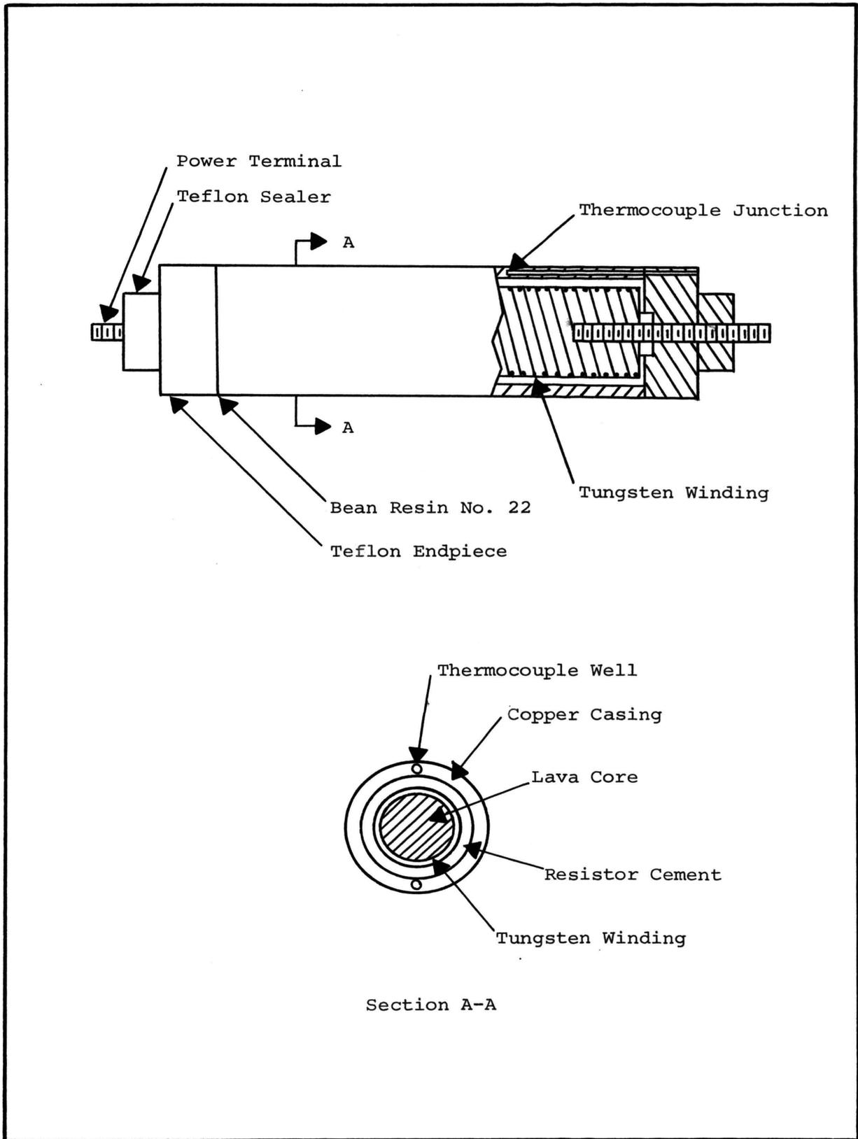
Figure 2. Heat Transfer Element
