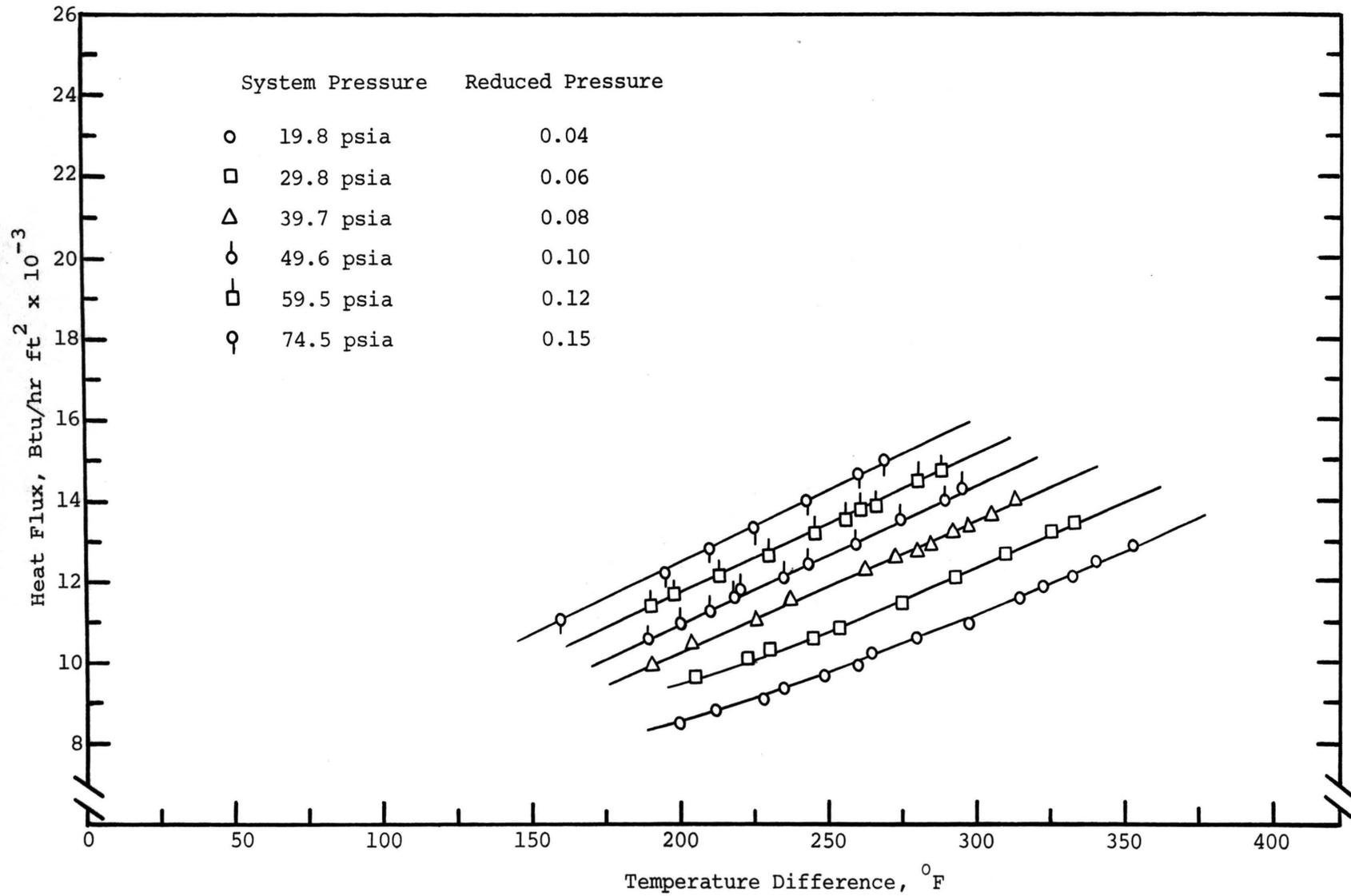
Figure 5. Film Boiling Results for Freon 113, 0.75 Inch Surface
