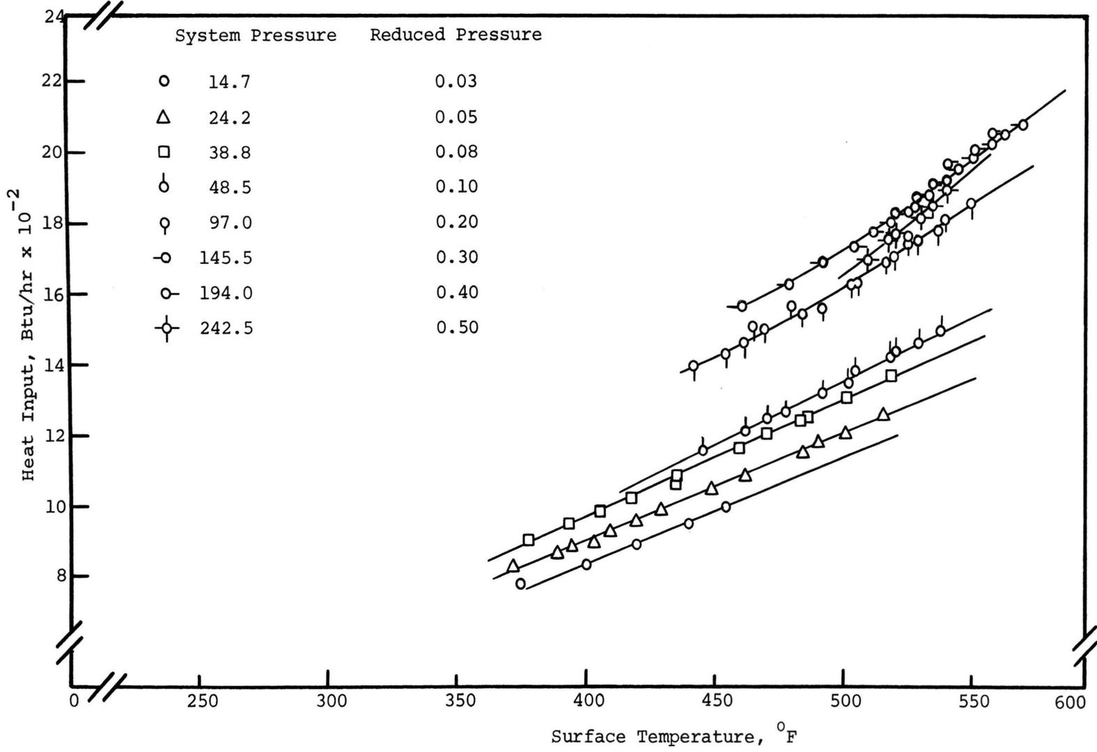
Figure 13. Film Boiling of n-Pentane as a Function of Surface Temperature, 1.00 Inch Surface
