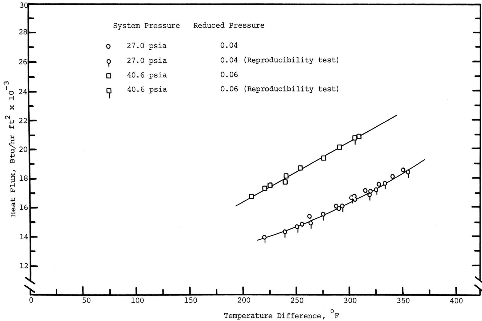
Figure 11. Film Boiling Results for Cyclopentane, 0.75 Inch Surface
