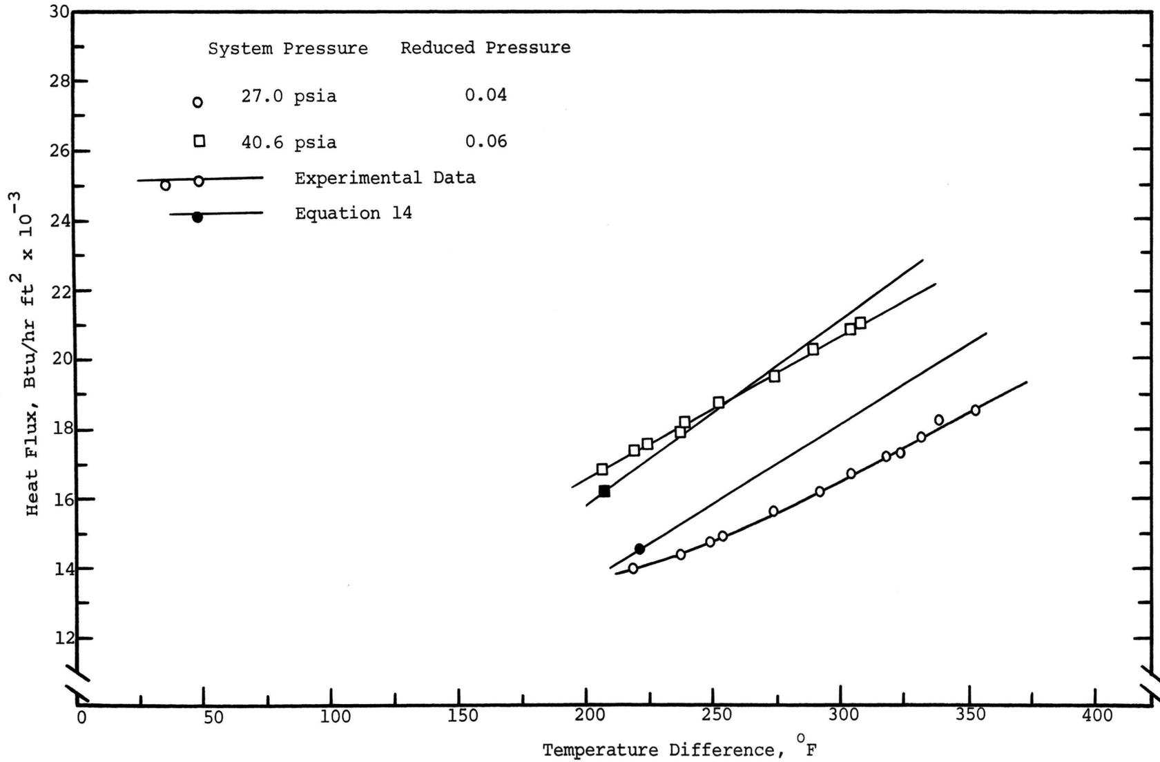
Figure 33. Film Boiling Comparison with Equation 14, Cyclopentane, 0.75 Inch Surface
