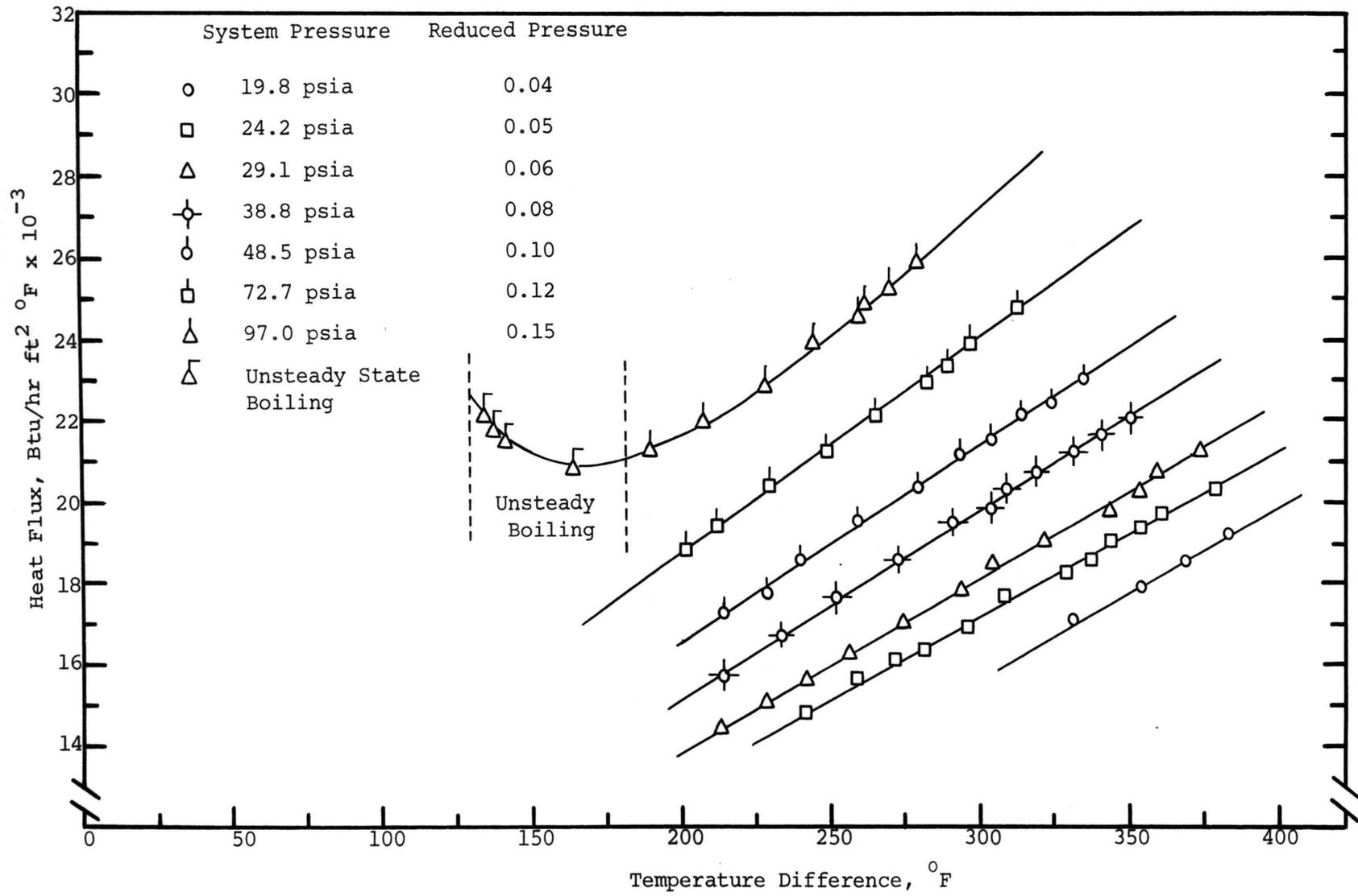
Figure 9. Film Boiling Results for n-Pentane, 0.55 Inch Surface
