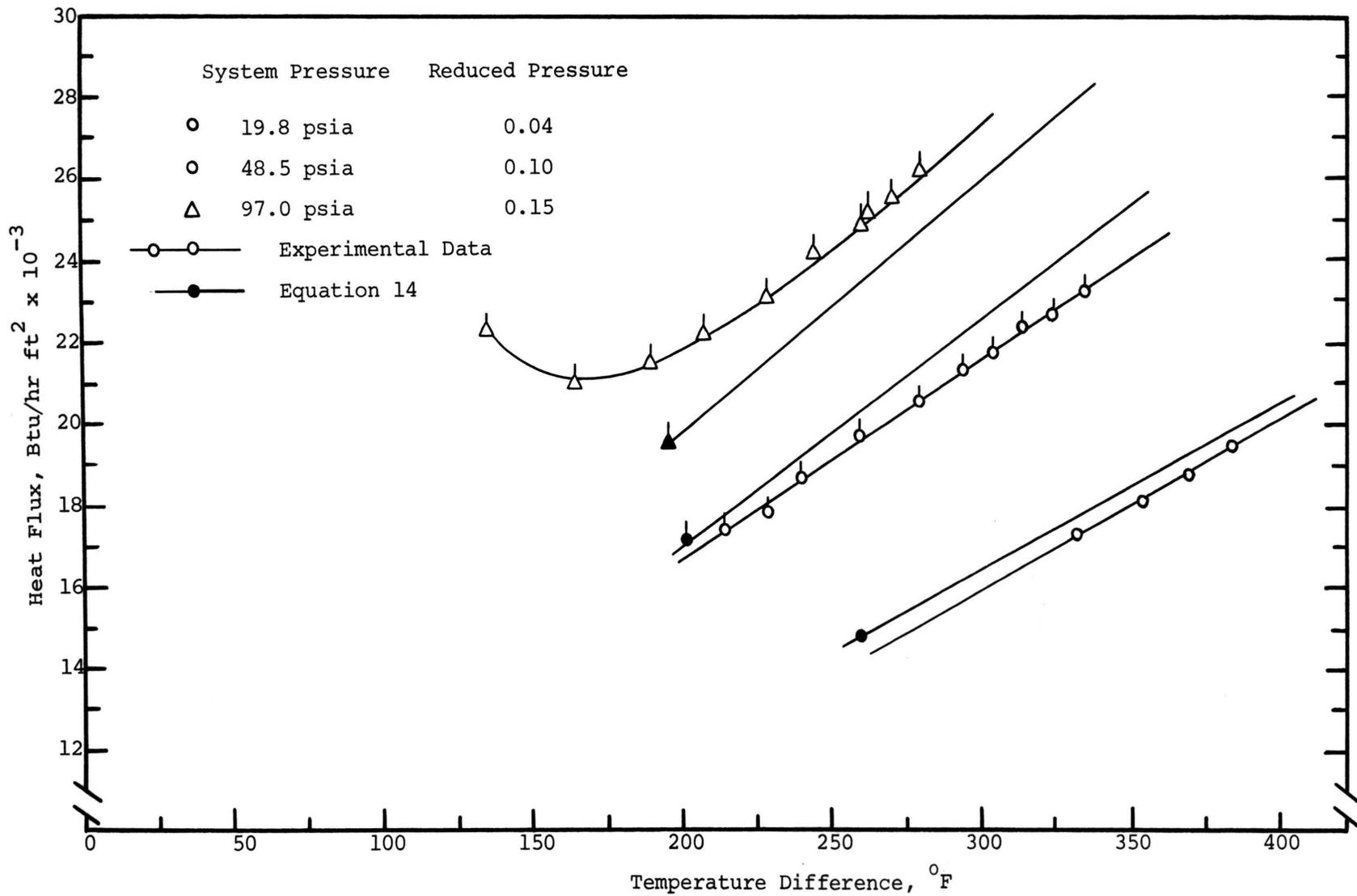
Figure 26. Film Boiling Comparison with Equation 14, n-Pentane, 0.55 Inch Surface
