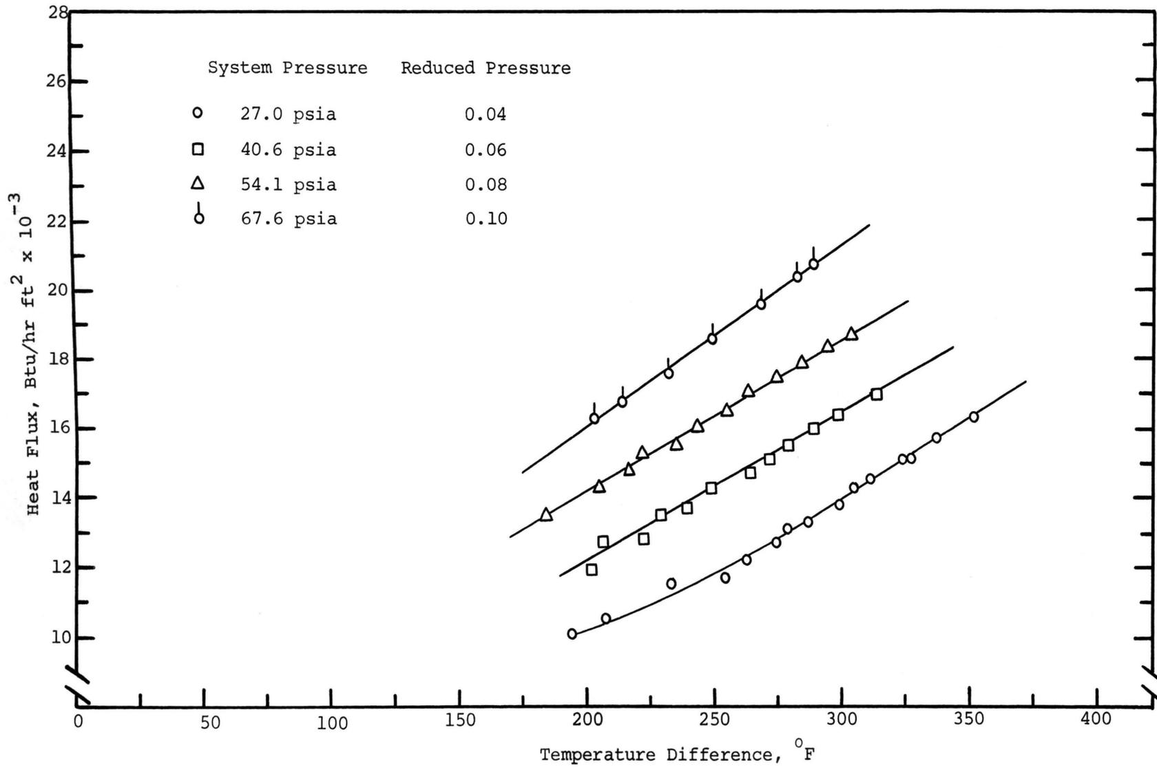
Figure 10. Film Boiling Results for Cyclopentane, 1.00 Inch Surface
