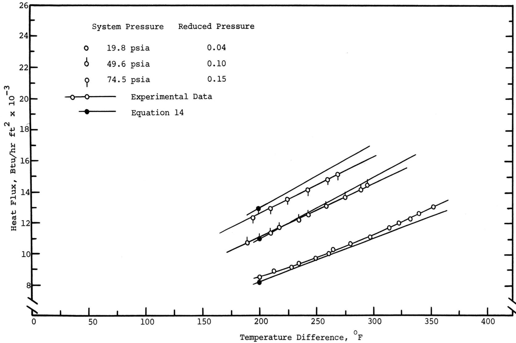
Figure 29. Film Boiling Comparison with Equation 14, Freon 113, 0.75 Inch Surface
