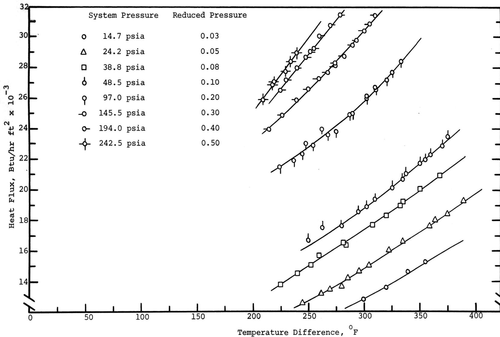
Figure 7. Film Boiling Results for n-Pentane, 1.00 Inch Surface
