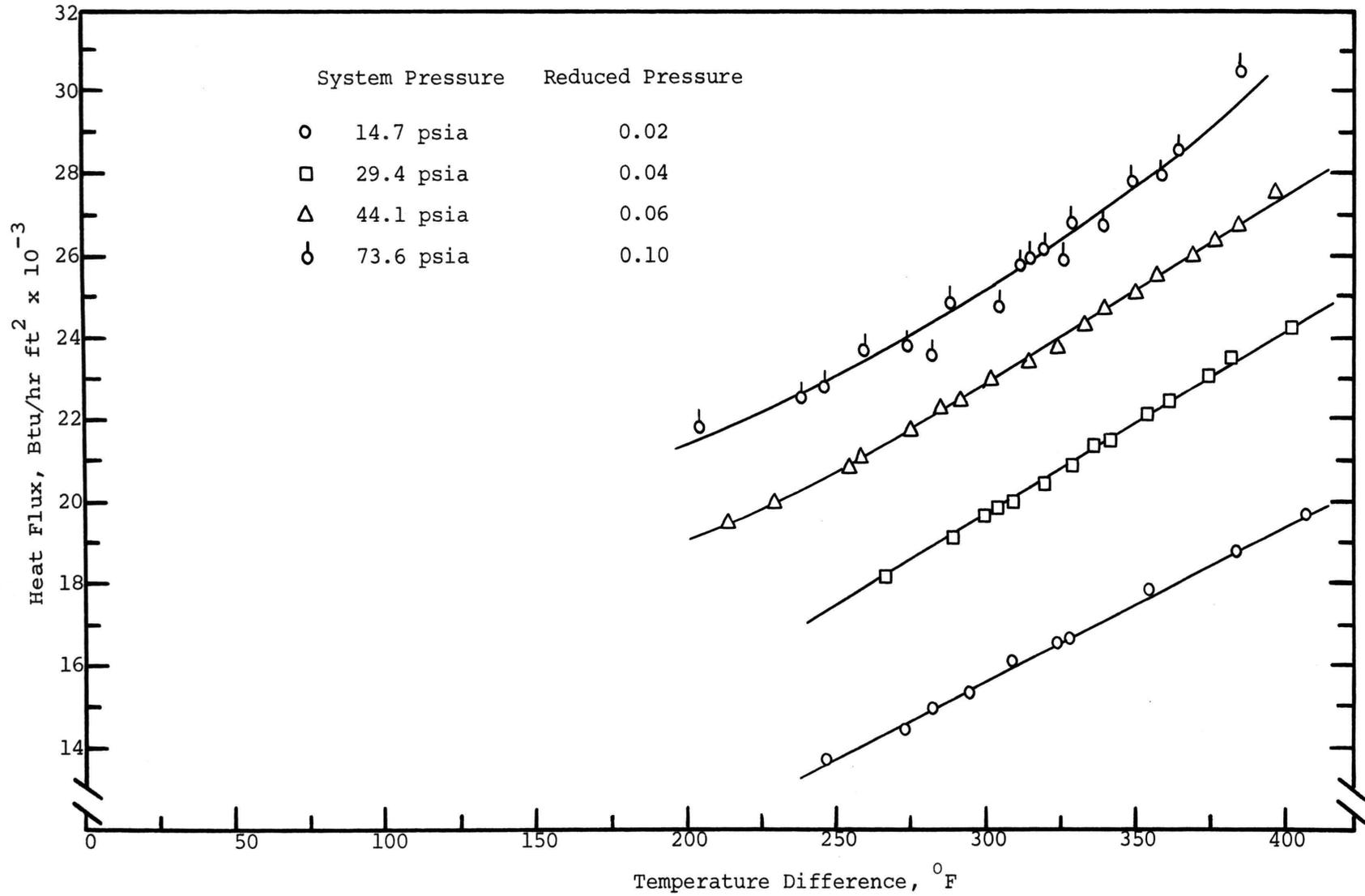
Figure 12. Film Boiling Results for Benzene, 1.00 Inch Surface
