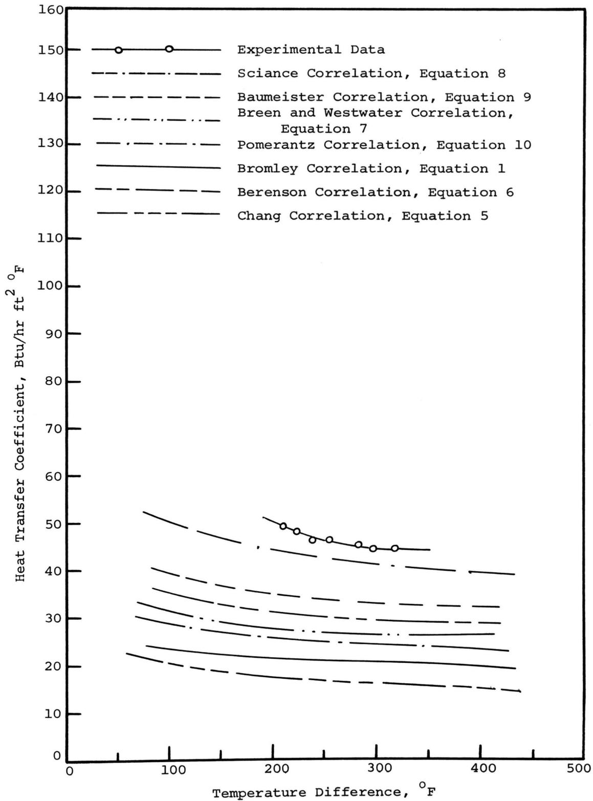
Figure 21. Comparison of Film Boiling Correlations, Freon 113, 49.5 psia, 1.00 Inch Surface
