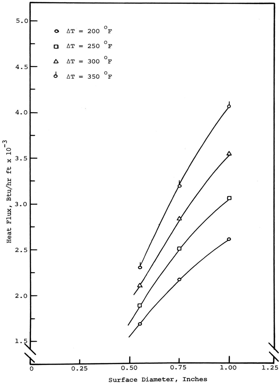
Figure 16. Film Boiling as a Function of Surface Diameter, Freon 113 at 49.6 psia
