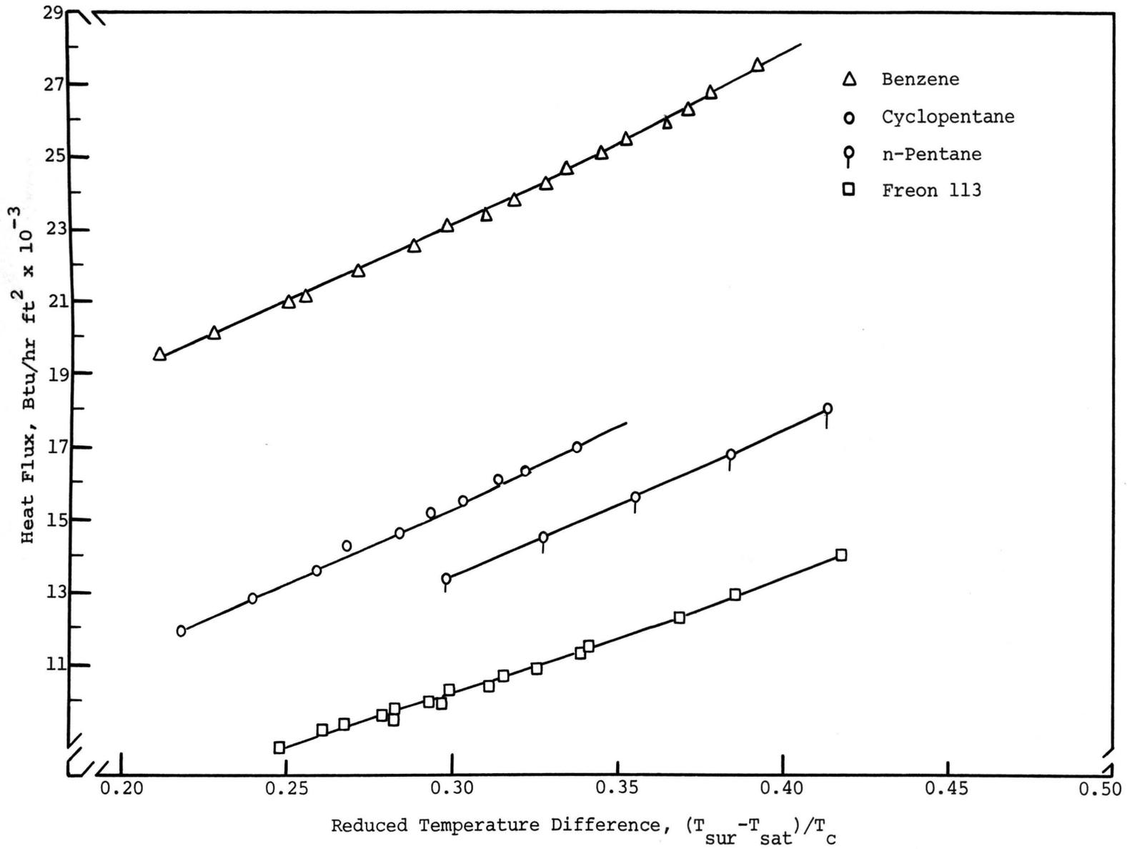
Figure 14. Film Boiling as a Function of Reduced Temperature Difference, 1.00 Inch Surface, 0.06 Reduced Pressure
