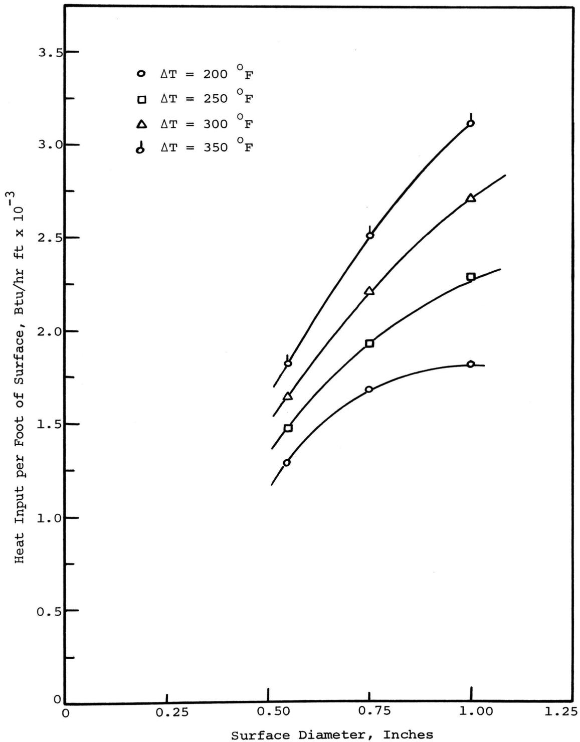
Figure 15. Film Boiling as a Function of Surface Diameter, Freon 113 at 19.8 psia
