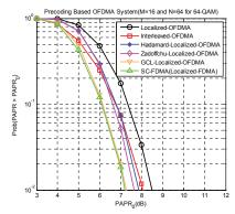
Figure 9. CCDF of L-OFDMA conventional, I-OFDMA conventional, WHT Precoder Based OFDMA, Zadoff-Chu Precoder Based L-OFDMA, GCL Precoder Based L-OFDMA and SC-FDMA (LFDMA) for 64-QAM.
