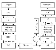
Figure 3. Block diagram of Precoding based OFDMA system.
