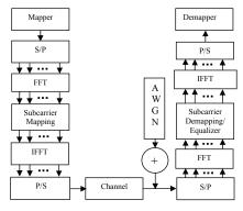
Figure .2. General Block diagram of Single Carrier System
