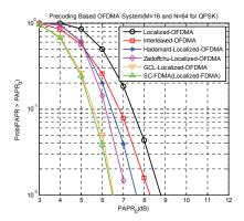
Figure 7. CCDF of L-OFDMA conventional, I-OFDMA conventional, WHT Precoder Based OFDMA, Zadoff-Chu Precoder Based L-OFDMA, GCL Precoder Based L-OFDMA and SC-FDMA (LFDMA) for QPSK
