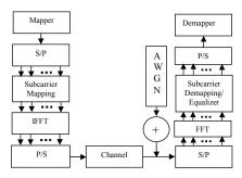
Figure 1. General Block diagram of OFDMA system
