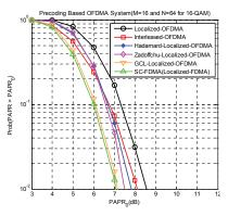
Figure 5. CCDF of L-OFDMA conventional, I-OFDMA conventional, WHT Precoder Based OFDMA, Zadoff-Chu Precoder Based L-OFDMA, GCL Precoder Based L-OFDMA and SC-FDMA (LFDMA) for 16-QAM.
