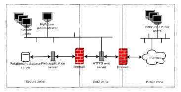
Figure 6: Network Architecture for MyFuture Deployment
