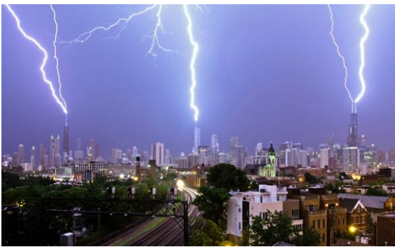
Figure 3: Simultaneous lightning strikes to three tall buildings in Chicago [4]
