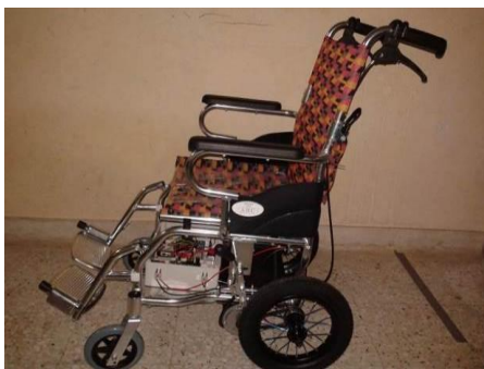
Figure 4: Voice control wheelchair
