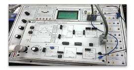
Figure 3: KL-75001 Electrocardiogram ECG Module and KL-72001 Biomedical Measurement System Module board
