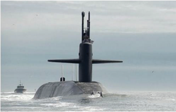
Figure 1: The two front control surfaces of this Ohio-class ballistic missile nuclear submarine USS Tennessee are seen attached to its conning tower [8]
