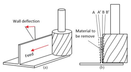
Figure 1: Un-cut materials in machining thin-wall feature
