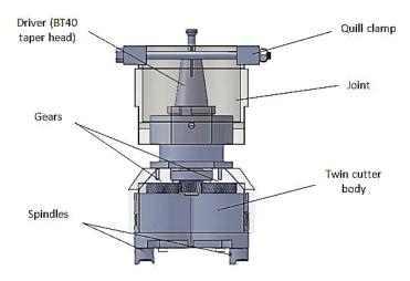
Figure 3: Principle of twin cutter machining technique
