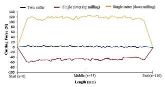
Figure 11: Cutting force exerted in Fx direction for single cutter technique and twin cutter technique
