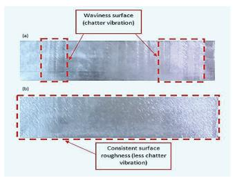
Figure 12: Machined surface condition for (a) Single cutter (b) Twin cutter technique
