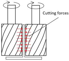
Figure 2: Act of cutting force in twin cutter machining technique
