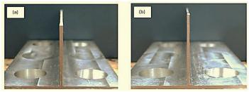
Figure 10: Wall thickness after machining with (a) Single cutter technique and (b) Twin cutter technique
