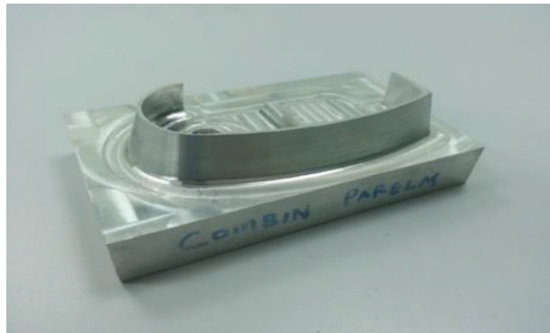
Figure 5: Combin Parelm strategy gives the best surface finish
