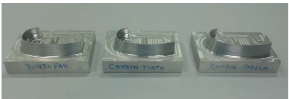
Figure 3: Machined parts of flank milling strategies
