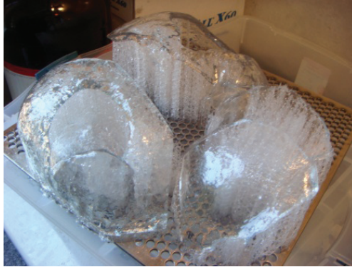
Figure 7: Completed SLA parts before the cleaning process
