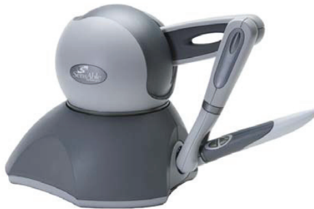
Figure 1: Phantom Omni Basic device with 6 degree-of-freedom
