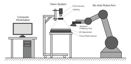
Figure 1. The general system design of the spolishing robot.
