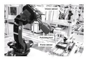
Figure 2. Implementation of the polishing robot system
