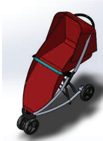
Figure 4: Redesign of front bar for sweet Cherry SCR8 stroller
