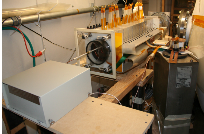
Figure 2.3. Missouri Plasmoid Experiment Mk.II segmented single-turn coil design along with integrated probe assembly.
