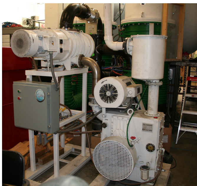
Figure 2.6. 2-stage roughing pump backing of high vacuum diffusion pumps. Upper left: roots-blower. Lower-right: rotary-vane pump.
