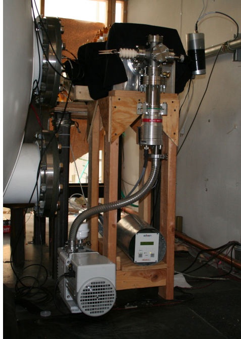
Figure 2.7. Small pump combination located downstream of the Mk.II device (in the upper-right corner of Figure 2.3).
