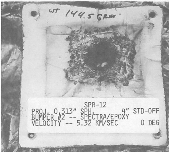
Fig. 7. Spectra/epoxy intermediate bumper, test no. SPR-12.
