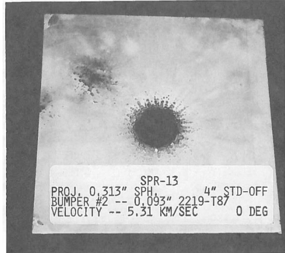
Fig. 9. Aluminum intermediate bumper, test no. SPR-13.
