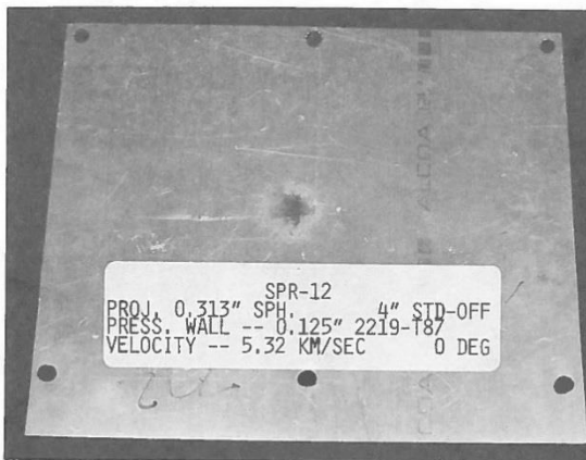
Fig. 8. Aluminum pressure wall plate, test no. SPR-12.
