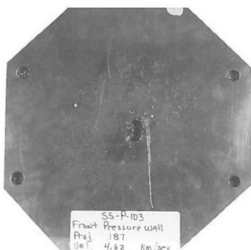
Fig. 2c. Pressure Wall Plate, Front (Test No. 103)
