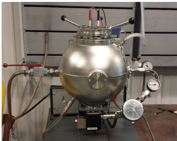
Fig. 4. Siwek 20-Liter Sphere used for testing
