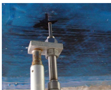
Figure 3-8 Installation of LVDT
