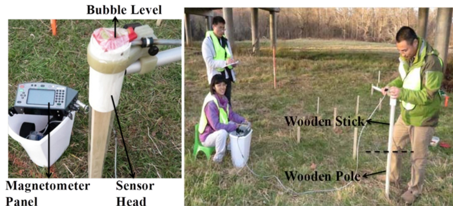
Figure 4.10. Magnetometer setup and operation.
