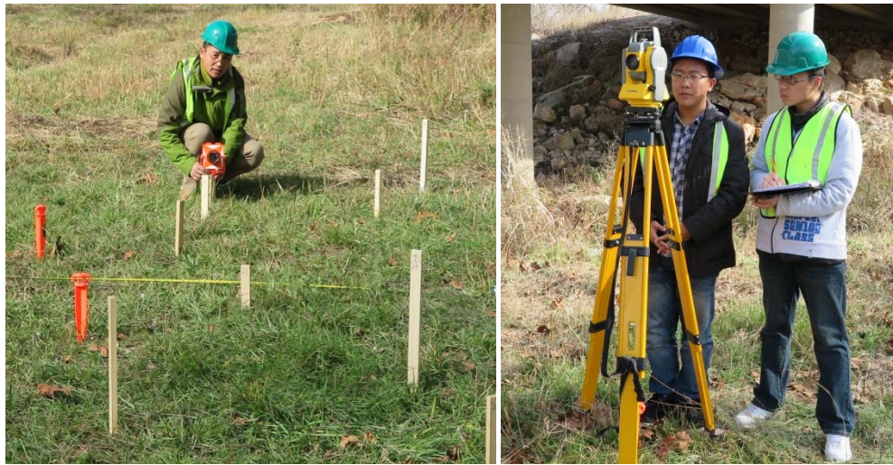
Figure 4.8. Total station and prism for positioning.
