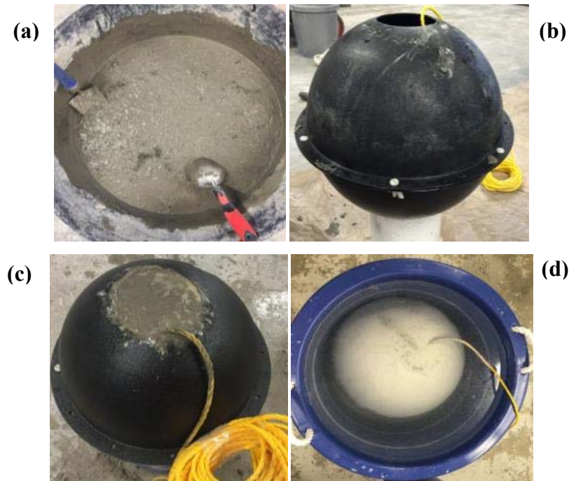
Figure 2.11. Four-step fabrication of concrete encasement: (1) preparing fiber reinforced concrete, (b) placing an APUS into concrete and mold, (c) filling the mold with concrete, and (d) curing the concrete encasement in water for 14 Days.
