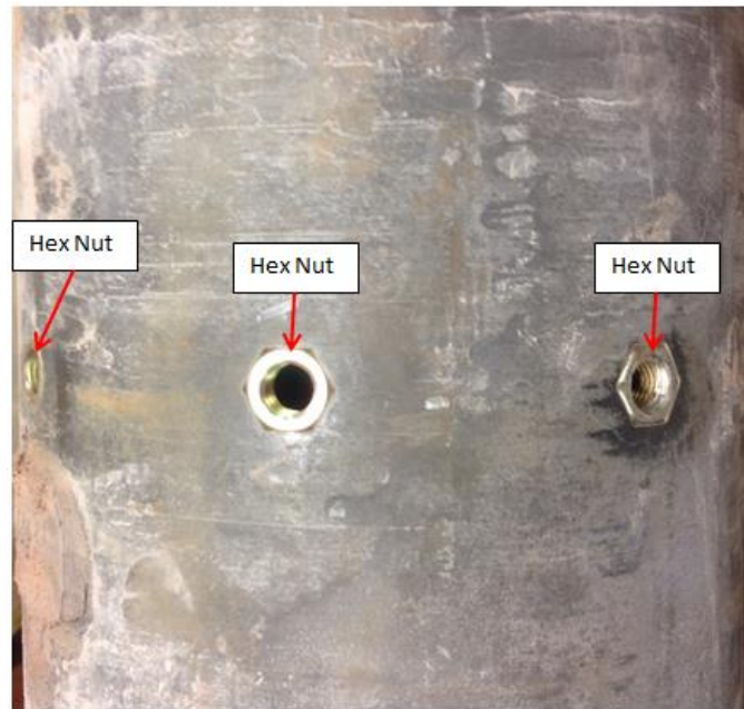
Figure E.3. The hex nuts inserted into the cylinder wall of Pipe 1 to serve as the sensor mounts.
