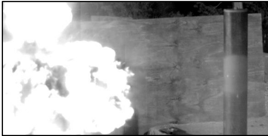
Figure 4.5. Single charge (Pipe 2) pipe stand setup for phantom side view, signature sensor pointed parallel to the bunker.
