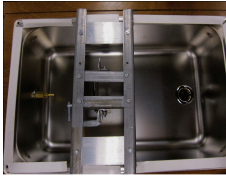
FIGURE 1: Schematics and photograph of the authors' test rig to assess nanofluid wear.
