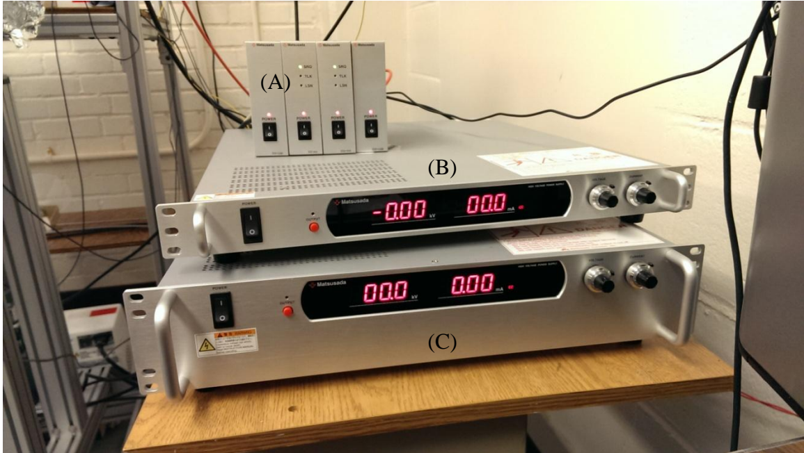
Figure 4.2. Power supplies used for electron extraction and acceleration. (A) Computer control interface, (B) 5 kV power supply, (C) 120 kV power supply.
