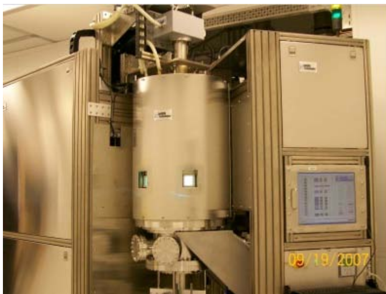
Figure 2.5. 915 MHz large area MPCVD system used for UNC films growth at the Center for Nanoscale Materials, Argonne National Laboratory [23].
