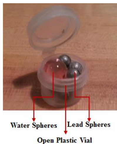
Figure 3.22. Photograph of Phantom Representing Low and High Atomic Number Materials
