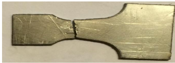
Figure 3. The failure crack at the specimen's lower cross section area.
