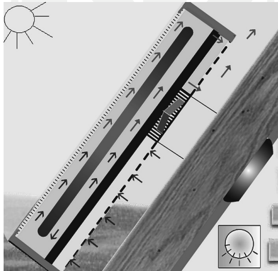
Fig. 4. A working diagram of a SolarVenti sun collector during a cooling cycle [7]
