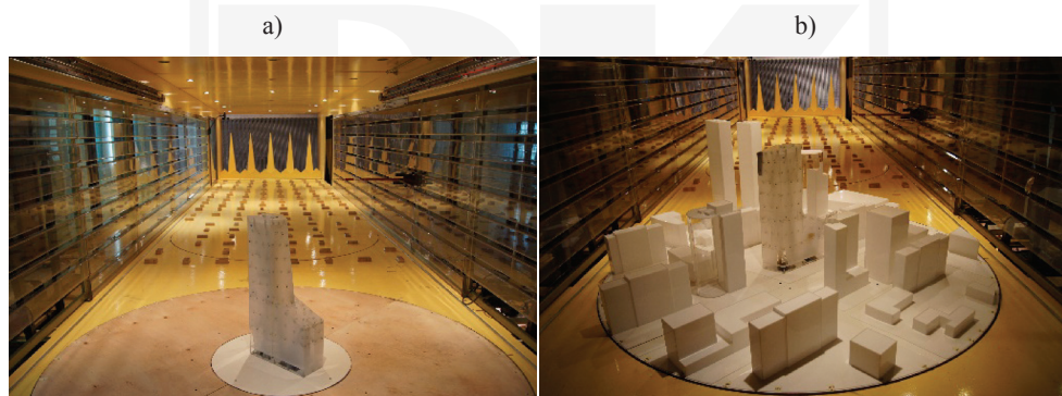
Fig. 2. Measuring configurations: a) a non-interference configuration; b) an interference configuration
