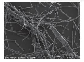
Fig. 1. SEM microphotograph of flax fibers
