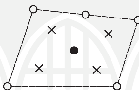
Fig. 2. Approximation and integration between nodes: \circ – nodes j , \times – Gauss stations, \bullet – equilibrium equations and yield condition application point
