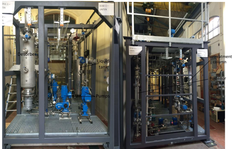
Fig. 4 Photos of the lower module (left) and of the upper module (right)
