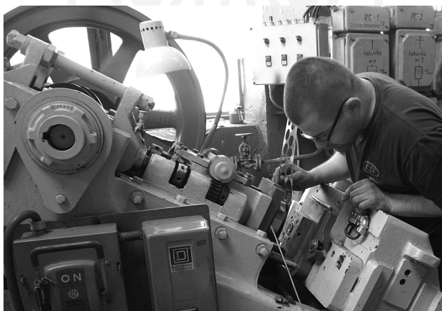
Fig. 3. View of the experimental system for measuring pressing forces
