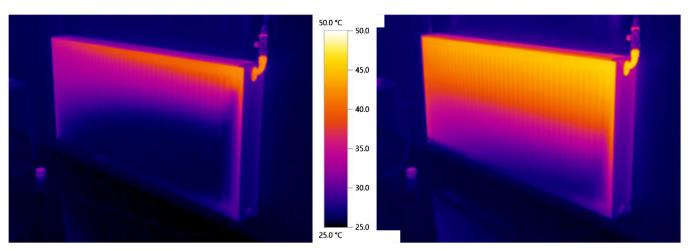
Fig. 2. Thermographic images during heat-up. Left) after 5 minutes. Right) after 8 minutes.
