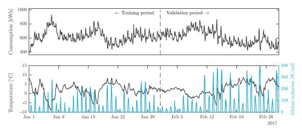
Fig. 6. Aggregated DH-consumption of urban district (only the 159 buildings marked in green in Fig. 5) and weather data for the training period (January 2017) and the validation period (February 2017).
