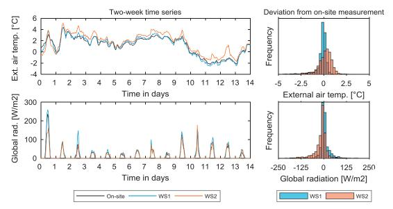
Fig. 2. Comparison of on-site measurements and the two weather stations.
