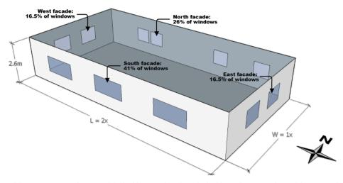
Fig. 1. Geometric model used for approximating the areas of the building envelope from the building's floor area. The model assumes a length/width ratio of 0.5, a room height of 2.6 m, and distribution of windows as depicted.
