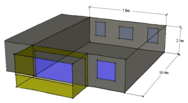
Fig. 5. Test case geometry as modeled in EP.
