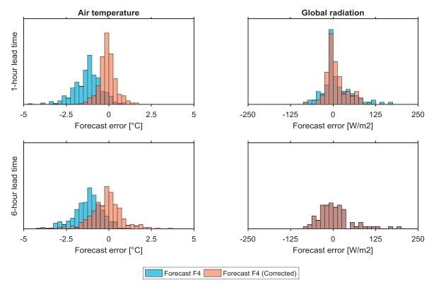
Fig. 7. Impact of forecast bias corrections of air temperaturte and global solar radiation on short-term forecast errors. Top: 1 h lead time. Bottom: 6 h lead time.
