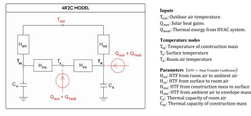
Fig. 1 Model structure and coefficient nomenclature.
