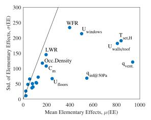
**Fig. 6.** Graphical presentation of the results of the Morris sensitivity analysis using r=500 trajectories and p=5 levels. The absolute mean elementary effects are plotted against the standard deviation of the elementary effects (20 uncertain model input parameters). The ten most influential parameters are named. The line represents values for which  $\sigma(EE) = \mu(EE)$ .
