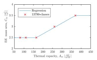
Fig. 7. Regression used to couple the thermal capacity  $(C_m)$  and the effective mass area  $(A_m)$  of ISO 13790.
