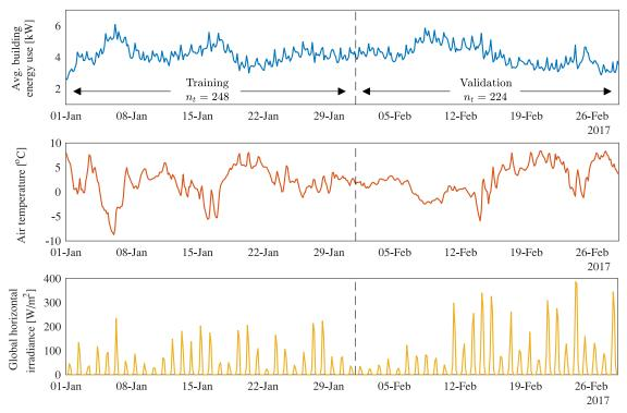
**Fig. 3.** Measured time series data. Top: Averaged building energy use for all  $n_b = 50$  within-sample training buildings. Middle: Outdoor air temperature. Bottom: Global horizontal irradiance. Only data from the training period was used for calibration.
