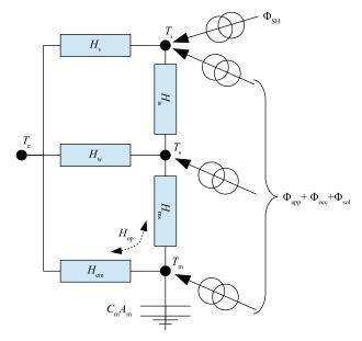
**Fig. 5.** Space heating model. Modified version of the network presented in ISO 13790:2008. The area of the building elements A is used to transform resistances R into heat transfer coefficients H = A/R.
