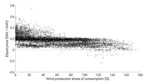
Fig. 1. The effect of wind power production on day-ahead electricity prices in the DK1 area. Source: Nord Pool, 2015 data.
