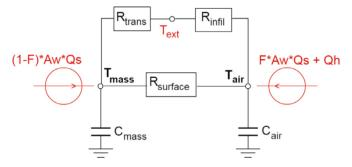
Fig. 5. RC-network of the physics-based 3R2C-model used in the MPC scheme of each apartment.
