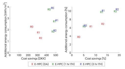
**Fig. 5.** Economic performance of the algorithm and effect on consumption aggregated for all apartments. Left (a) absolute differences from reference, right (b) relative to the reference.
