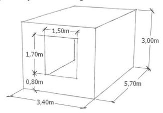
Figure 1. Geometry of the EnergyPlus model
