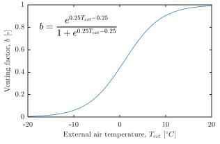
Fig. 4. Model for external temperature-dependent manual venting.
