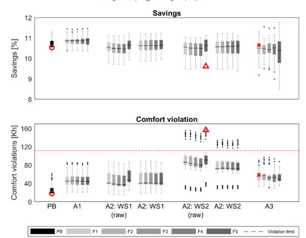
**Fig. 10.** Energy savings and comfort violations from the MPC simulations of the different scenarios (see Table 1) using weather forecasts from different locations (see Fig. 1). Red symbols refer to specific simulations shown on Fig. 9. (For interpretation of the references to color in this figure legend, the reader is referred to the web version of this article.)
