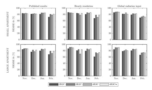
Figure 9 Impact of the used dataset on the NRMSE fits of the resulting models evaluated on the validation data. The top/bottom row presents results for the small/large apartment, while each column refers to the dataset (published, hourly or global radiation) used for identifying model parameter.
