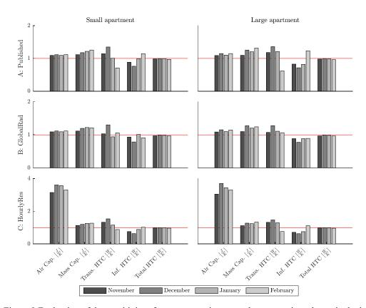
Figure 8 Evaluation of the sensitivity of parameter estimates to the assumptions drawn in the initial analysis. Normalized parameter values relative to their white-box estimate (red line). Rows 1, 2 and 3 present the estimates obtained with data using 1) transmitted solar data with 1-minute resolution (from the paper), 2) global radiation with 1-minute resolution, and 3) transmitted solar with hourly resolution.
