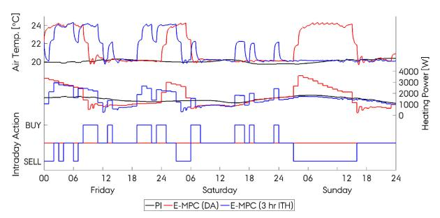
Fig. 4. Example period of both upward and downward regulation in the Retrofit2 building.
