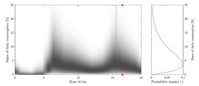
Fig. 9. Contours of marginal prior distributions for both DHW profiles (workdays/weekends). The contour at each x-coordinate depicts the marginal distribution for that specific hour of the day – see highlighted hour.
