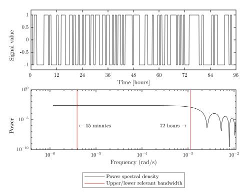
Figure 4 Full-length PRBS signal and its power spectrum. Relevant bandwidth as per [46, 47]. Only part of the signal is shown – length of full signal is approx. 28 days.
