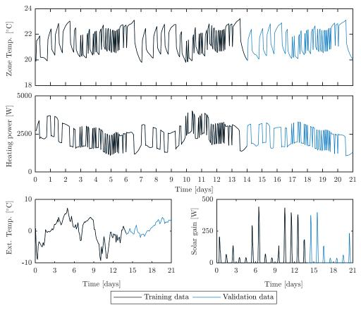
Figure 6 The Input-output used for parameter identification. The data was simulated with an EnergyPlus model containing two apartments. For readability, the data is here presented as hourly values.
