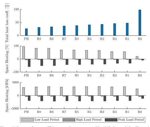
Figure 11 Impact of energy efficiency on the energy quantities shifted to periods of low grid load. Top) Total heat loss coefficient of each building, middle/bottom) the amount of space heating consumption that was shifted to/from each period.
