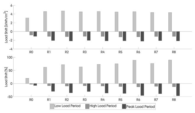
Fig. 8. Accumulated load shift of centralized E-MPC for all retrofit scenarios compared to the baseline PI control. Top: Absolute load shift. Bottom: Relative load shift.
