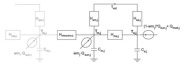
Fig. 2. Illustration of the model structure for apartment j and adjacent apartments i.
