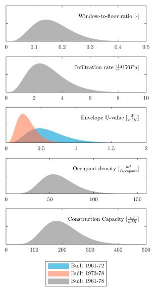
**Fig. 8.** Prior-specification of building-specific parameters  $(\theta_B)$ . The prior of the WFR (top graph) is specified as a Beta distribution, while all other priors where specified as Gamma distributions.
