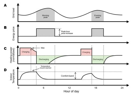
Fig. 14. Principle of the price-based demand response scheme evaluated in this study.
