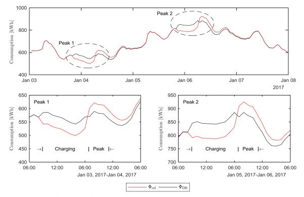
Fig. 17. The response of the case buildings obtained by solving the optimization problem of Eqs. (11a)–(11e) including the constraints of Eqs. (12a) and (12b), and imposing the optimal increase in price indicated in Fig. 16 during peak periods.
