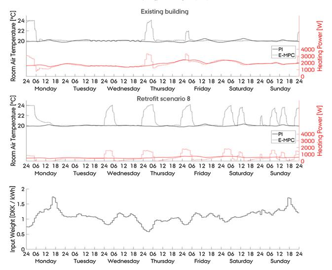
**Fig. 6.** Simulation results for apartment 7 for the existing building (top) and retrofit scenario 8 (middle) using a PI controller and E-MPC scheme, respectively, during the period December 7–14, 2015. The bottom chart shows the energy price (input weight c) during the same period.
