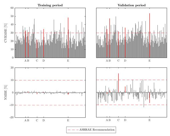
Fig. 10. Performance metrics CVRMSE and NMBE for each building model parameterized with the MAP parameter estimates. Time series of the five highlighted buildings (A–E) are presented in Fig. 11.
