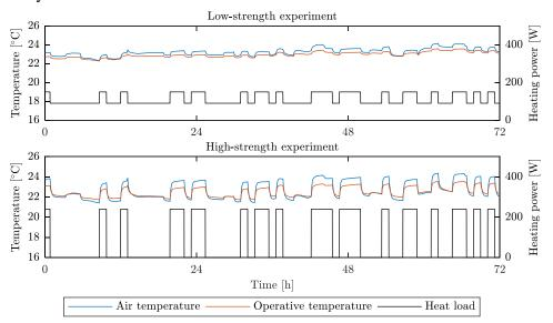
Fig. 4 Comparison of low- and high-strength experiments. Top: PRBS1, Bottom: PRBS4.
