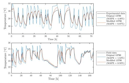
Fig. 3. Impact of the modification of the ISO 13790 model. The upper and lower graphs show simulation performance of the models when calibrated with experimental data and field data, respectively. The depicted models are parameterized with the maximum likelihood-estimates of the calibrated parameters.
