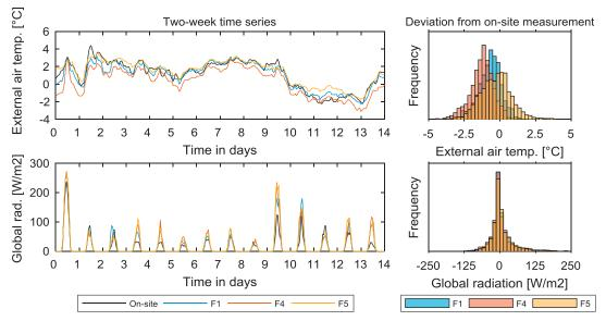
Fig. 3. Comparison of on-site measurements and forecast time-series for a period of two weeks.
