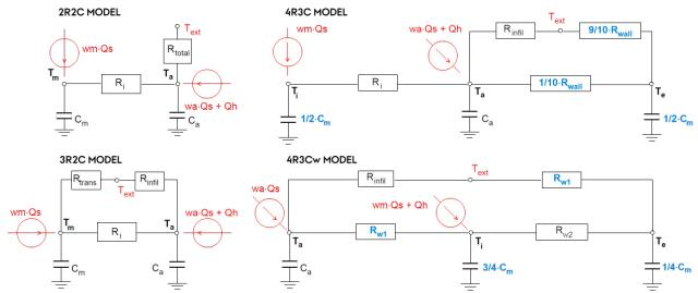
Figure 1 Model structures depicted as RC-networks. Red text denotes inputs, blue highlights the assumptions made for third order models.
