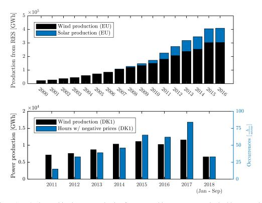
Figure 1 Top) The combined power production from renewable energy sources in the 28 EU member states, source: Eurostat. Bottom) Relationship between wind power production and the occurrence of negative prices in the DK1 day-ahead market region (source: Energinet).
