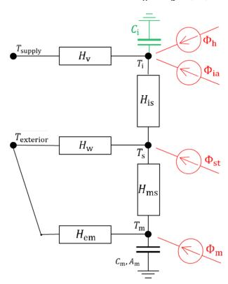
Fig. 2. Modified RC-network of the model used in ISO 13790's hourly method for calculating heat consumption. Green: modification, red: thermal loads.
