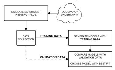
Fig. 3. System identification methodology (Hold-out cross-validation).
