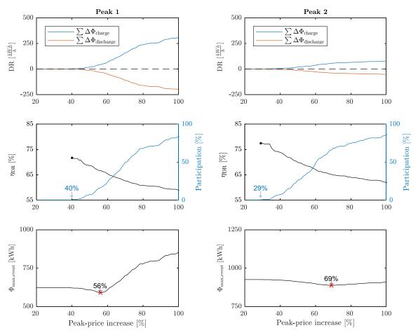
Fig. 16. Metrics describing the aggregated response of the buildings of the urban neighbourhood as a function of the increase in peak energy price. Top: pre-peak increase and on-peak reduction in consumption. Middle: load shifting efficiency and participation rate. Bottom: maximum consumption during event.
