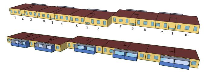
Fig. 1. Test case geometry as modelled in EnergyPlus with applied apartment numbering.
