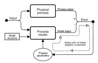
Figure 3 The principle of the family of prediction error methods in system identification.
