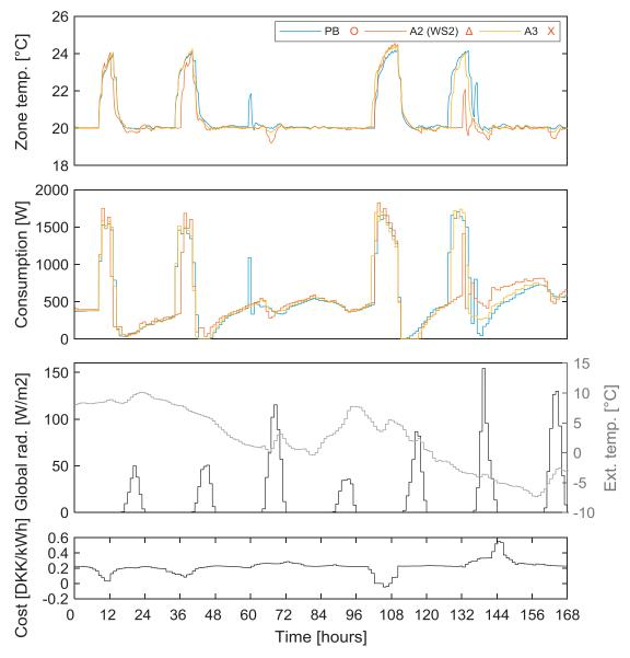
**Fig. 9.** Simulation data from an apartment controlled by the E-MPC-scheme for three weather source data scenarios. The red symbols in the legend refer to the results of Fig. 10. (For interpretation of the references to color in this figure legend, the reader is referred to the web version of this article.)
