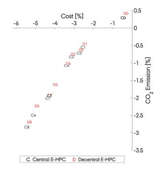
**Fig. 7.** Achieved cost and emission reductions for the centralized and decentralized E-MPC schemes relative to the PI controller for all simulations. The existing building is referred to with index 0 and the remaining numbers refer to the retrofit scenarios.
