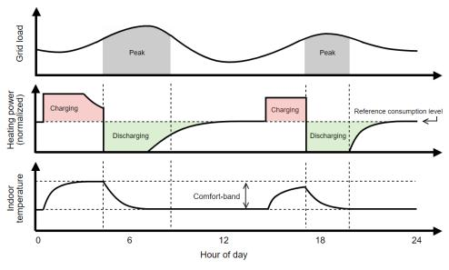
Figure 2 Principle in utilizing the structural thermal energy storage for demand response. Adapted from (P4).
