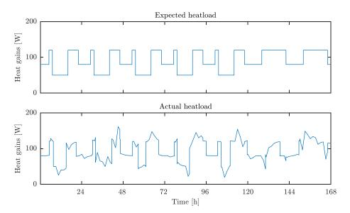
Fig. 2 Top: Expected heat load based on 24-hour static schedules. Bottom: Actual heat load, i.e. noise added to the static profile using the developed noise generator.
