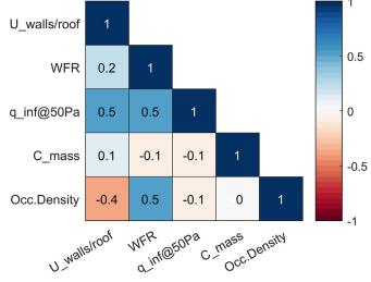
**Fig. 8.** Expected posterior correlation matrix,  $E_{post}[corr(\theta)]$ , of the five calibration parameters.
