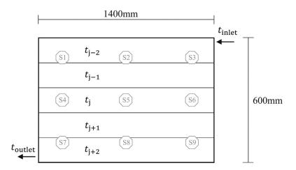
Fig. 1. Principle of the dynamic radiator model exemplified with  $N_S = 5$  horizontal sections with different temperatures t. The octagons mark the position of nine thermocouples (type K) used to measure the surface temperature.
