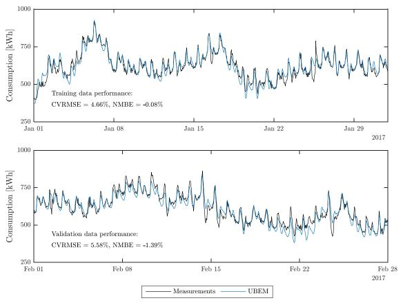
Fig. 13. Performance evaluation of the aggregated UBEM (159 buildings) on the dataset used for training (top) and on a previously unseen validation dataset (bottom). Both datasets are in hourly temporal resolution. CVRMSE and NMBE metrics for each period are indicated on each graph.
