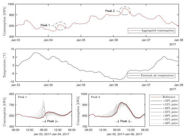
Fig. 15. Top: Aggregated heating consumption from the UBEM. Middle: External air temperature for the period. Bottom: The response of the UBEM obtained by solving the optimization problem of Eqs. (11a)–(11e) with different peak prices during the four hours of the peak period.
