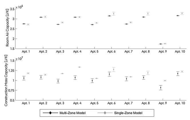
Fig. 3. Parameter estimations and standard deviation of the thermal capacity of the room air (top) and construction mass (bottom).
