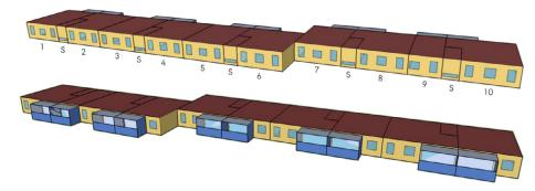
Fig. 4. Geometry of the 10-apartment building (3rd floor) used in the case study. Top: East façade. Bottom: West façade. (Illustration from [4]).
