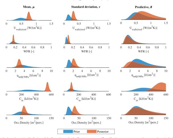
Fig. 7. Marginal prior and posterior distributions of the five archetype-level calibration parameters. The calibration parameter mean values  $\mu$  are shown in the left-hand column, their decoupled standard deviations  $\tau$  are shown in the middle column, and their predictive distributions are shown in the right-hand column.
