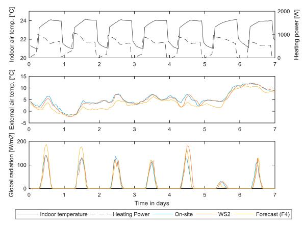
Fig. 6. One week of the hourly data used to identify grey-box models with three different sources for weather measurements.
