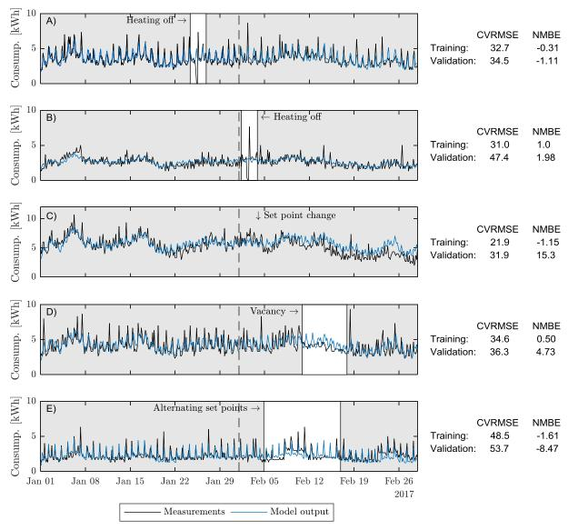
Fig. 11. Evaluation of individual building models that performed poorly in terms of CVRMSE/NMBE through comparison of time series. The dashed line separates the training and validation period. Time series of 3-hourly averages were used for readability. The NMBE and CVRMSE metrics are indicated next to the time series.
