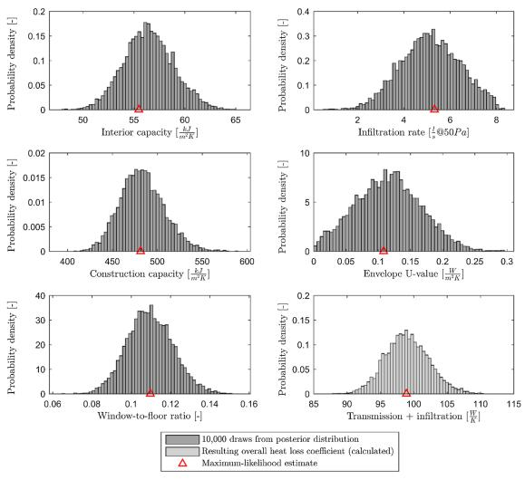
Fig. 18. Estimates of model parameter posterior distributions for the modified model structure. The estimates were obtained from the calibration using measurement data from a terraced house. Red markers indicate the ML-estimate of model parameters of the modified model used for the model-comparison of Fig. 3 (lower graph).
