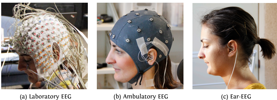
Figure 1.1: The evolution of EEG systems from conventional scalp EEG (a) to ambulatory (b) and wearable ear-EEG (c)
