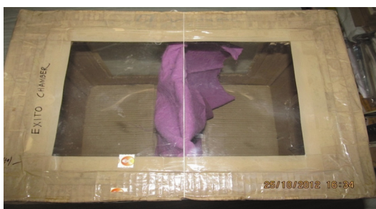
Fig. 1—Exito chamber [for mosquito repellency test]
