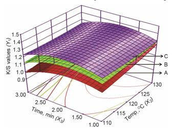
Fig. 3—Response surface plots for the *K/S* values ( $Y_1$ ) versus temperature and time at different GTA concentrations (A—10mL/L, B—20mL/L, and C—30mL/L)
