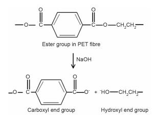
Fig. 2—Alkali hydrolysis of polyester<sup>15</sup>
