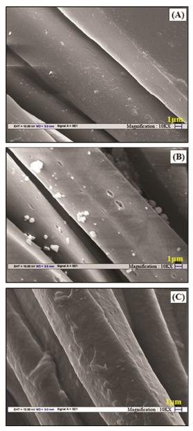
Fig. 1—SEM images of polyester (A) control, (B) alkali treated and (C) treated with alkali and 10g/L of sericin
