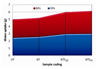
Fig. 5—In plane wicking values of untreated and sericin treated polyester fabric (UT–control, AT– alkali treated, ATS<sub>10</sub>–alkali and 10g/L sericin, ATS<sub>20</sub>–alkali and 20g/L sericin)
