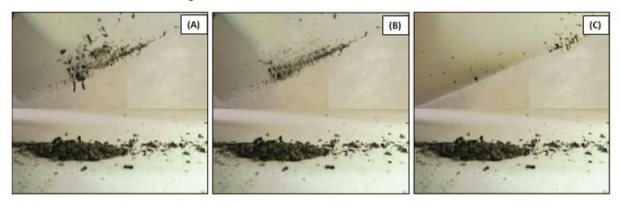
Fig. 7—Ash test for assessment of antistatic property (A) control, (B) alkali treated, and (C) alkali and 10g/L of sericin treated
