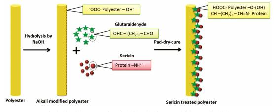
Fig. 4-Graphic representation of sericin application on modified PET using GTA
