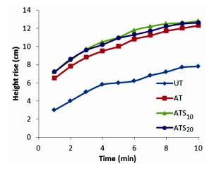
Fig. 6—Vertical wicking values of control and sericin treated polyester (UT–control, AT– alkali treated,  $ATS_{10}$ – alkali and 10gpl sericin,  $ATS_{20}$ – alkali and 20gpl sericin)
