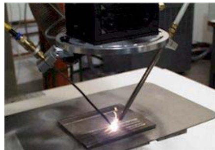
Figure 1: Laser Metal Deposition Manufacturing Process.
