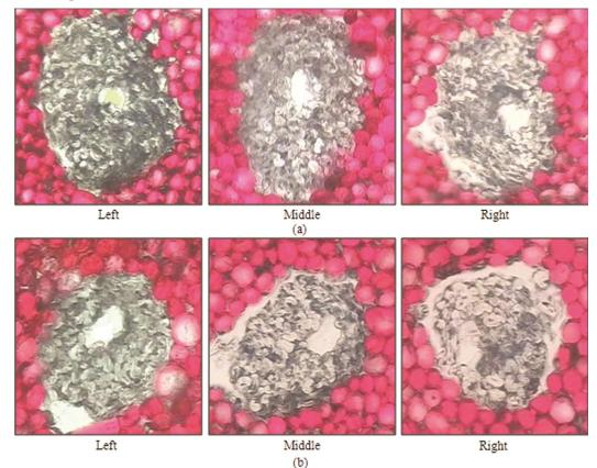
Fig. 3 — Cross-sections of (a) 29.2tex /44.4dtex and (b) 14.6tex/44.4dtex lattice apron compact siro-spinning core-spun yarns
