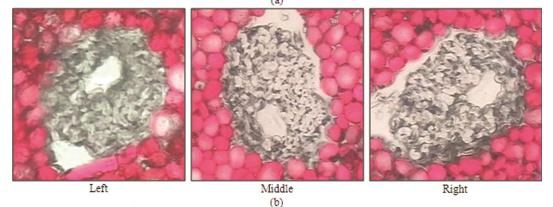
Fig. 4 — Cross-section of (a) 29.2tex /44.4dtex and (b) 14.6tex/44.4dtex complete condensed siro-spinning core-spun yarns
